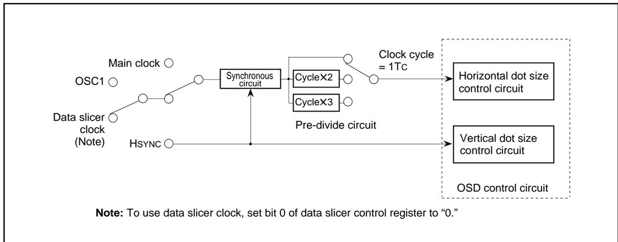
Fig. 64. Block Diagram of Dot Size Control Circuit
