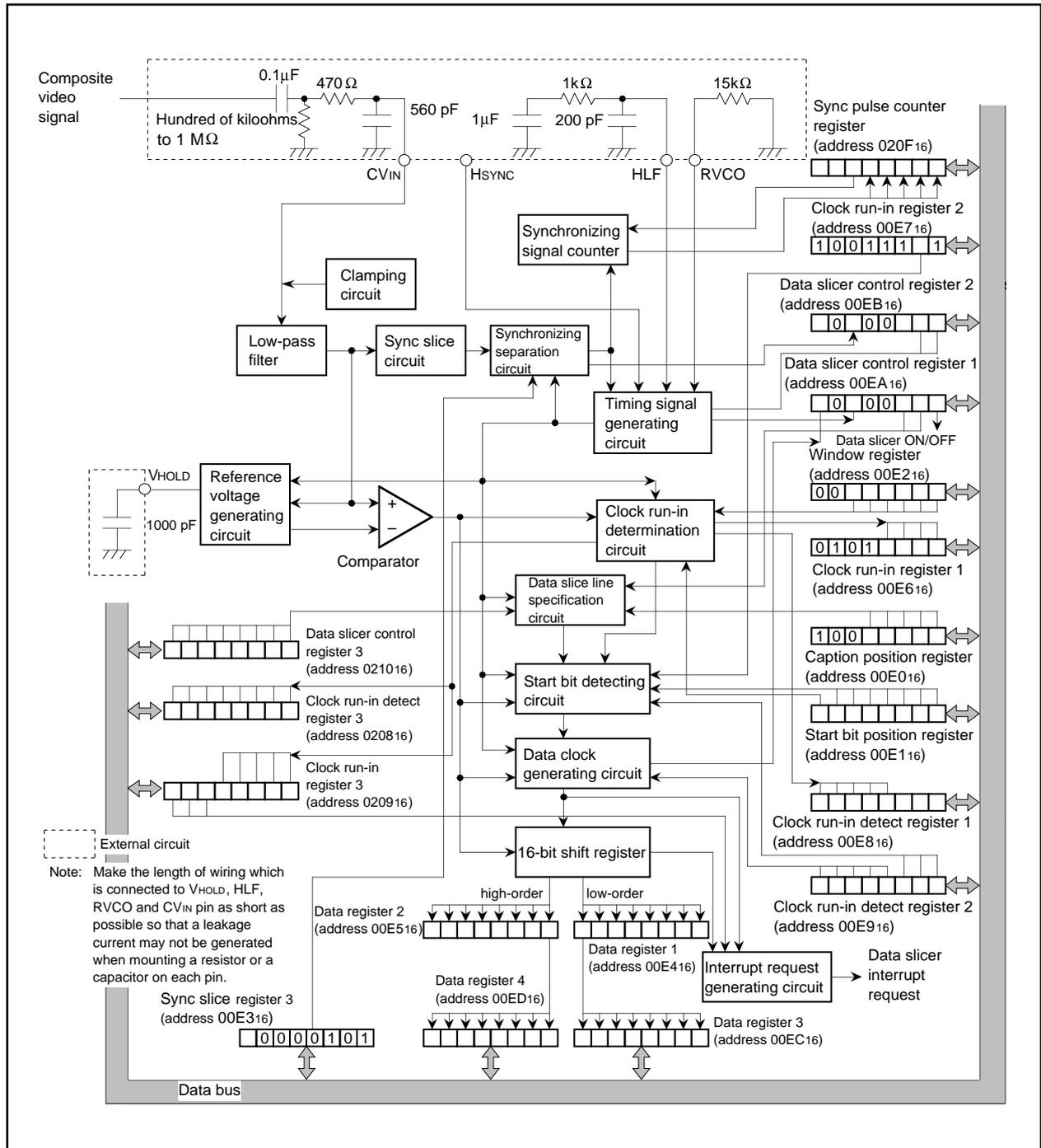
Fig. 25. Data Slicer Block Diagram
