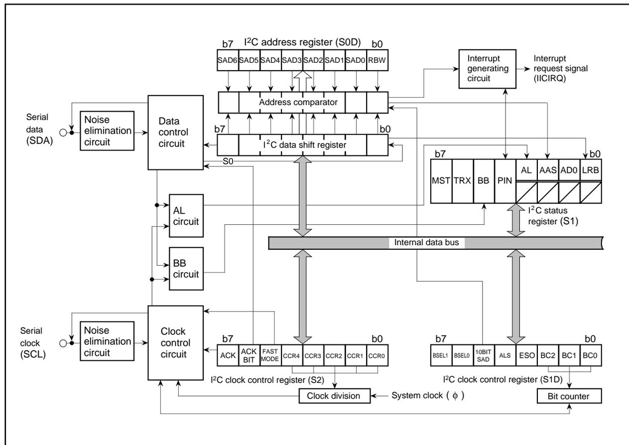
**Fig. 42. Block Diagram of Multi-master I<sup>2</sup>C-BUS Interface**
