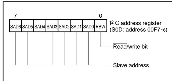
Fig. 43. I<sup>2</sup>C Address Register
