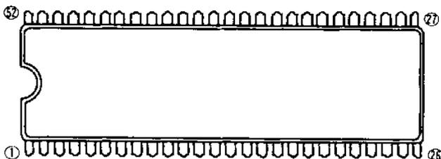
Note1: If the special mark is to be printed, indicate the desired layout of the mark in the upper figure. The layout will be duplicated as close as possible. Mitsubishi lot number (6-digit or 7-digit) and mask ROM number (3-digit) are always marked.
