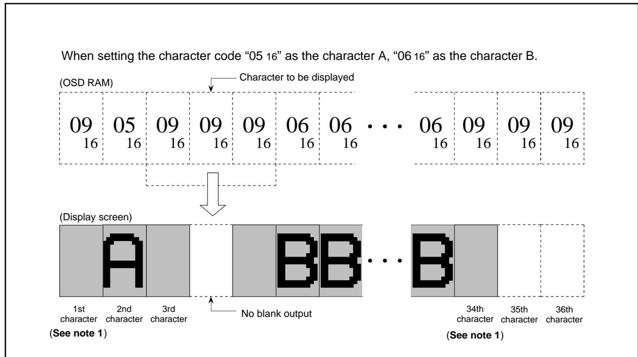
**Fig. 84. Display Screen Example of Automatic Solid Space**
