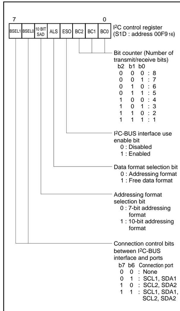
**Fig. 46. I<sup>2</sup>C Control Register**
