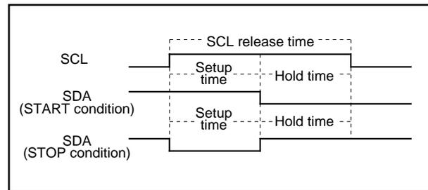
Fig. 51. START Condition/STOP Condition Detect Timing Diagram
