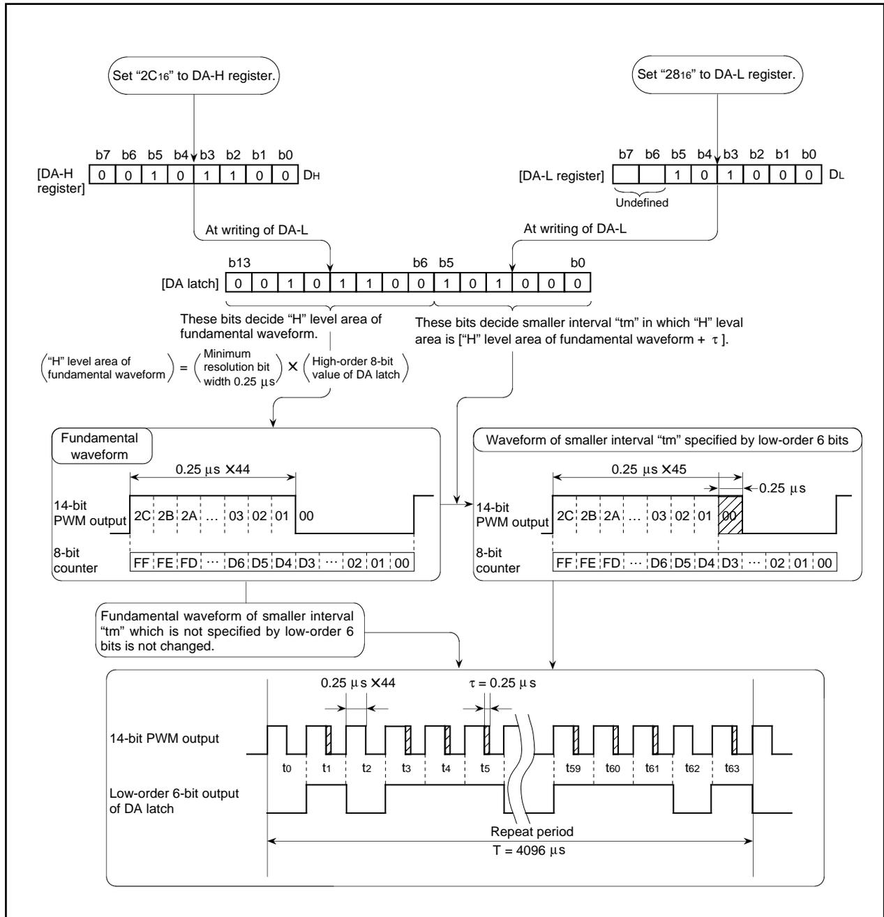
Fig. 19. 14-bit PWM Output Example ( $f(\text{XIN}) = 8\text{MHz}$ )
