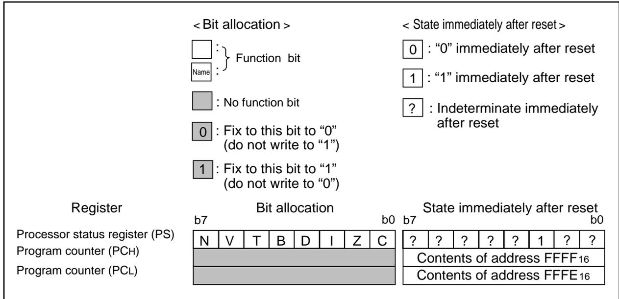
Fig. 9. Internal State of Processor Status Register and Program Counter at Reset
