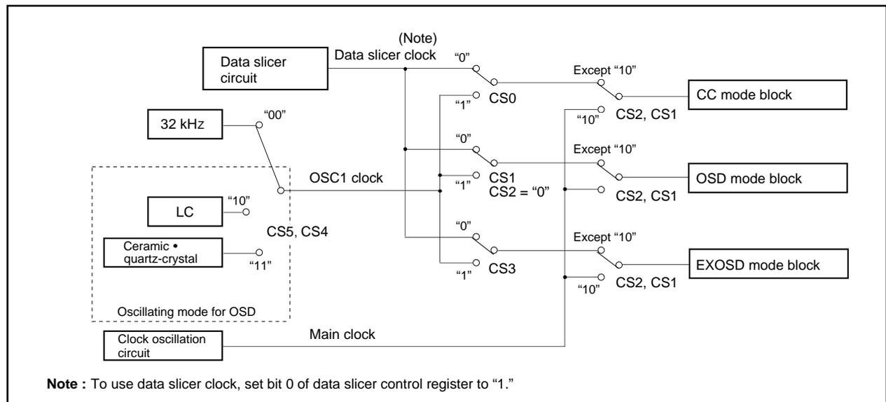
**Fig. 67. Block Diagram of OSD Selection Circuit**
