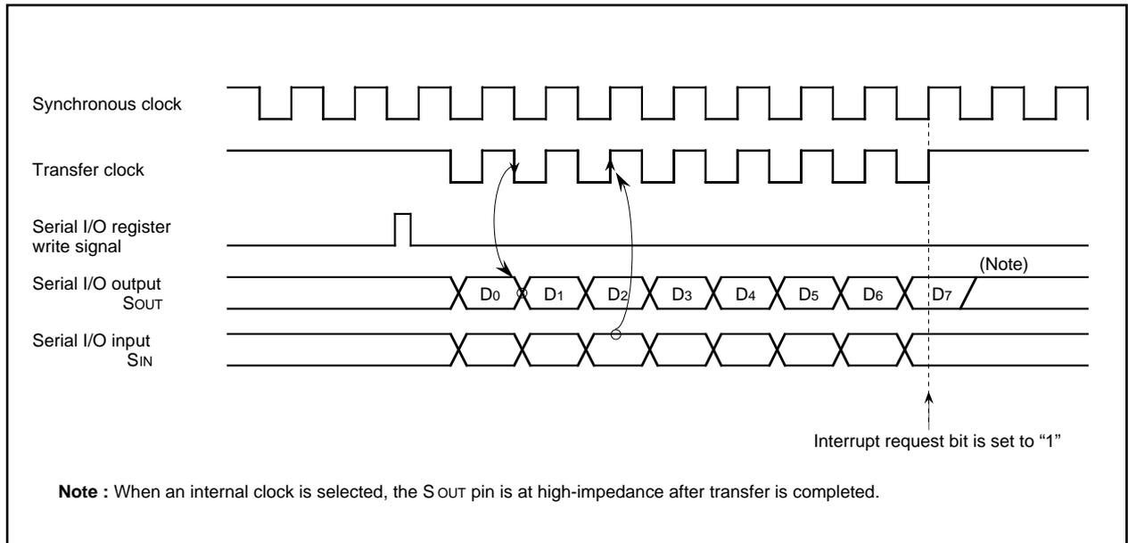
**Fig. 15. Serial I/O Timing (for LSB first)**
