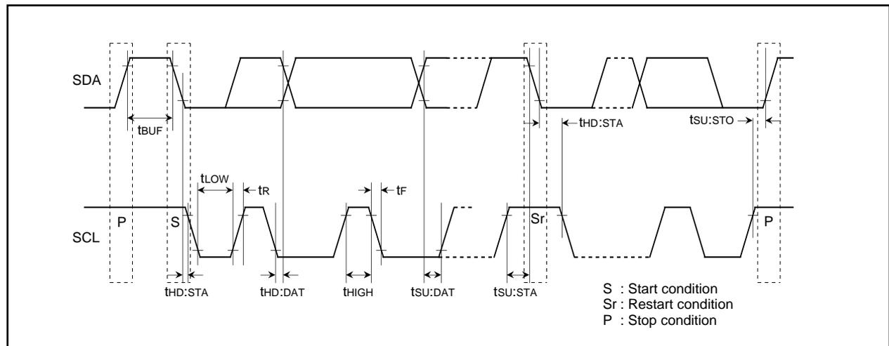
**Fig. 101. Definition Diagram of Timing on Multi-master I<sup>2</sup>C-BUS**
