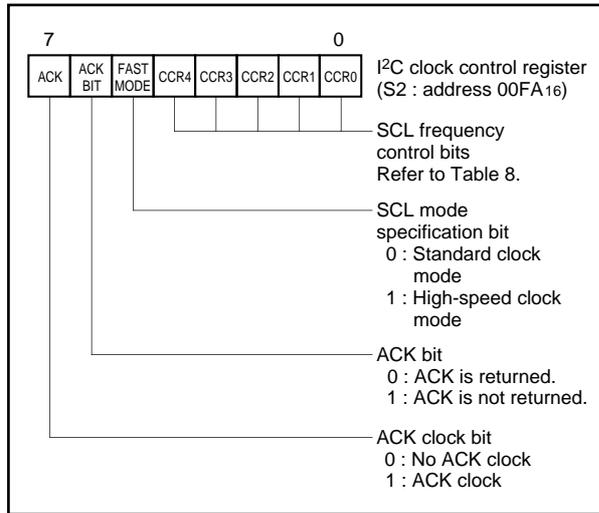
**Fig. 44. I<sup>2</sup>C Clock Control Register**
