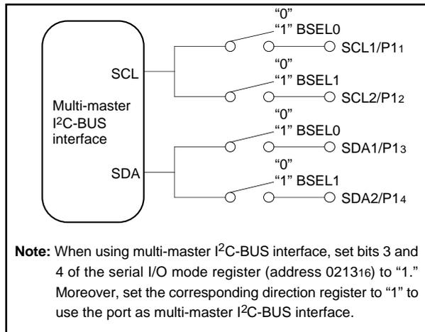
**Fig. 45. Connection Port Control by BSEL0 and BSEL1**
