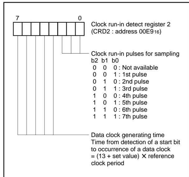
Fig. 34. Clock Run-in Detect Register 2
