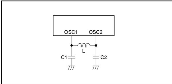
**Fig. 99. Display Oscillation Circuit**
