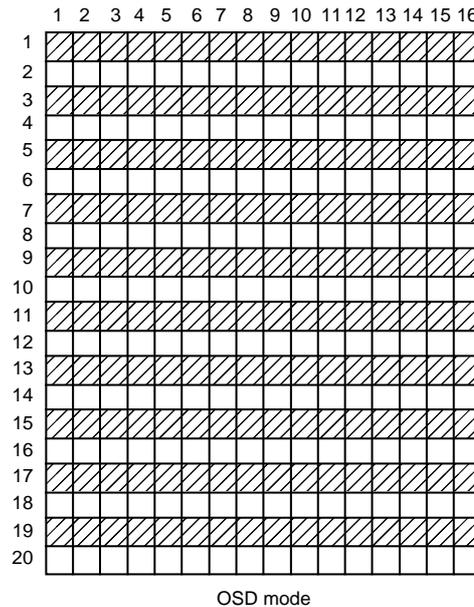
When the display dot line selection bit is "0," the "□" font is displayed at even field, the "▨" font is displayed at odd field. Bit 7 of the I/O polarity control register can be read as the field determination flag : "1" is read at odd field, "0" is read at even field.
