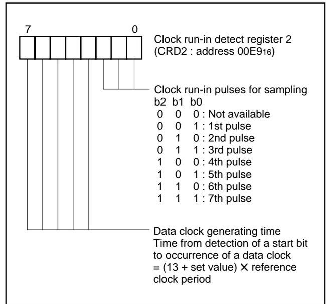
Fig. 31. Structure of clock run-in detect register 2
