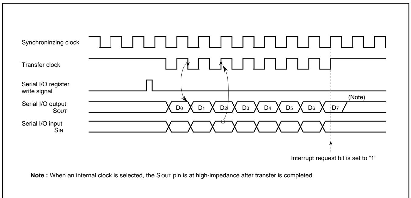
Fig. 13. Serial I/O timing (for LSB first)
