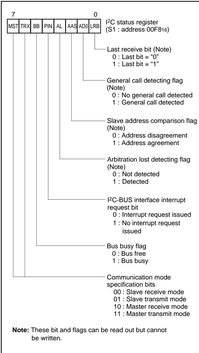
Fig. 44. Structure of I<sup>2</sup>C status register
