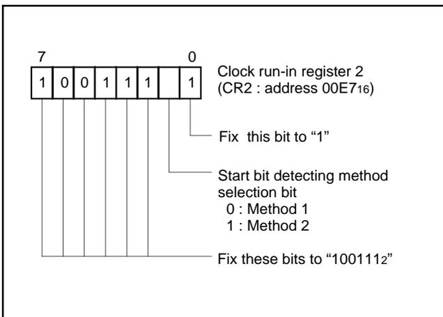
Fig. 30. Structure of clock run-in register 2
