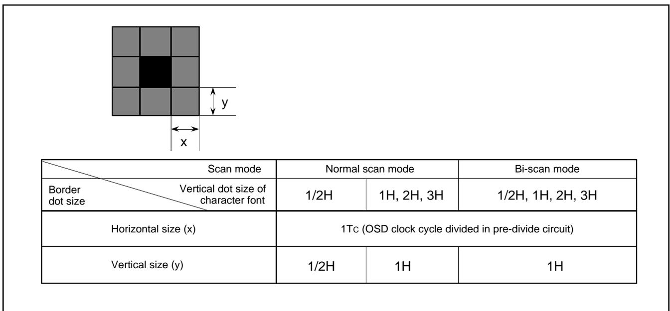
Fig. 74. Horizontal and vertical size of border
