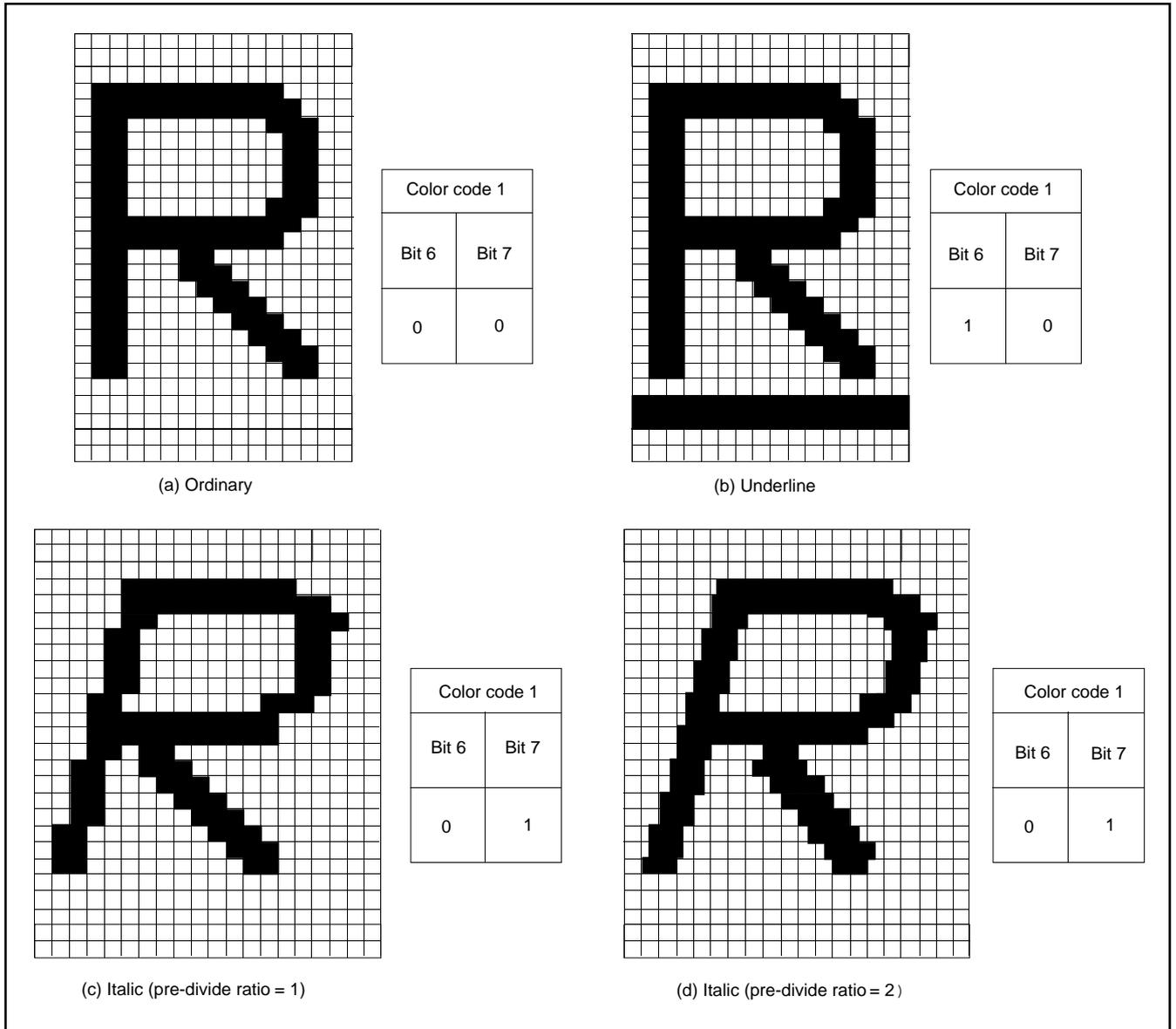
Fig. 71. Example of attribute display (in CC mode)
