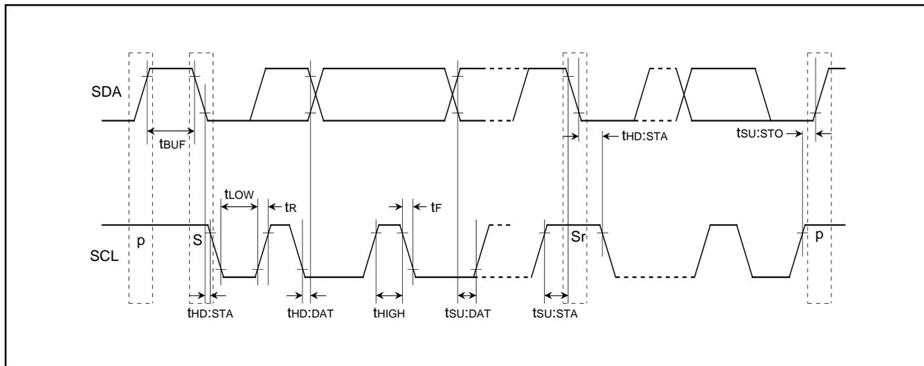
Fig. 100. Definition diagram of timing on multi-master I<sup>2</sup>C-BUS
