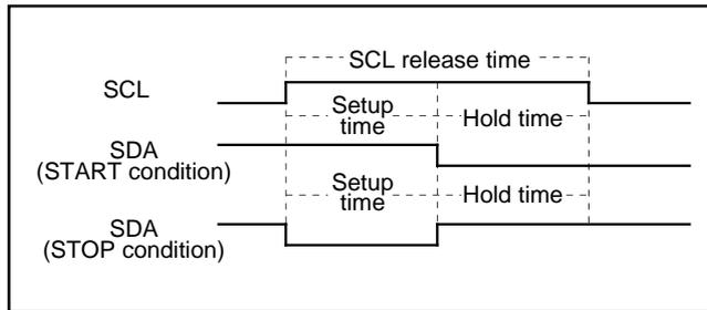
Fig. 48. START condition/STOP condition detecting timing diagram
