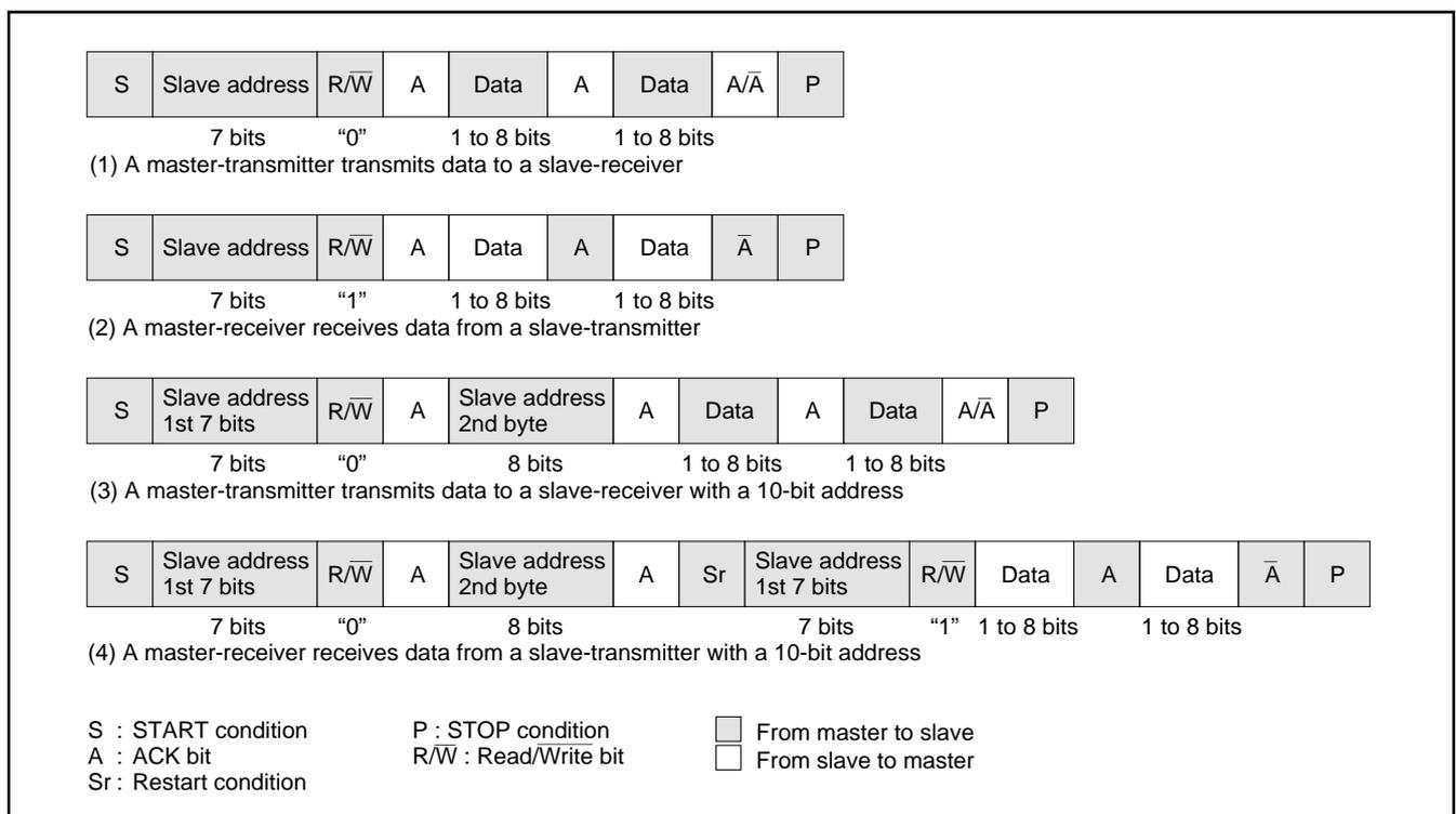
Fig. 49. Address data communication format
