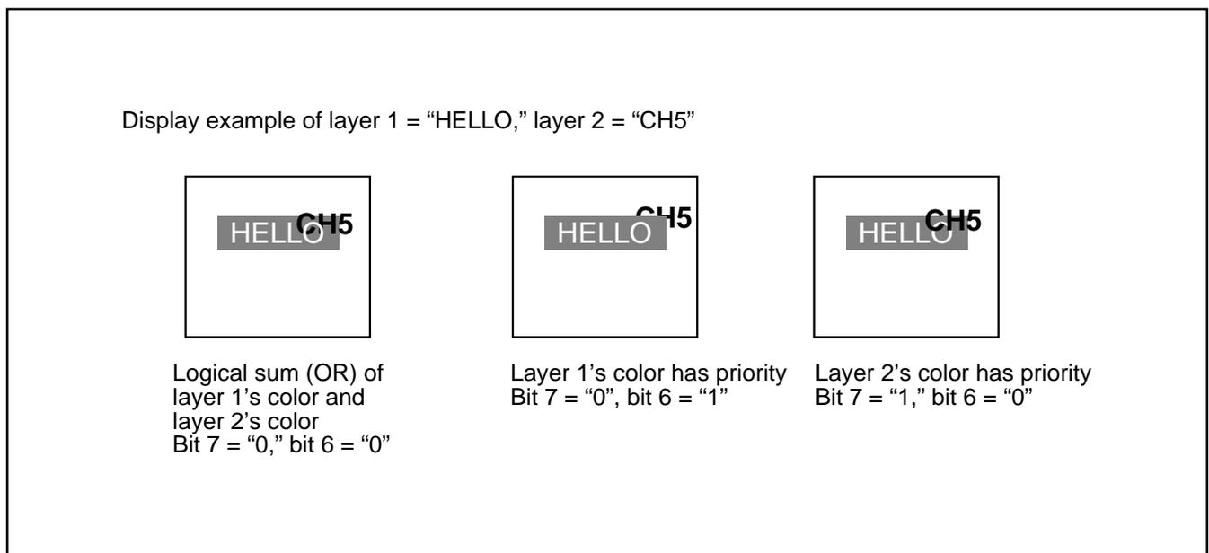
Fig. 55. Display example of dual layer OSD
