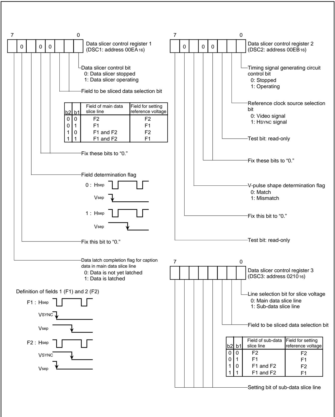
Fig. 23. Structure of data slicer control registers
