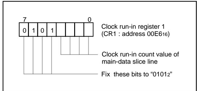
Fig. 33. Structure of clock run-in register 1
