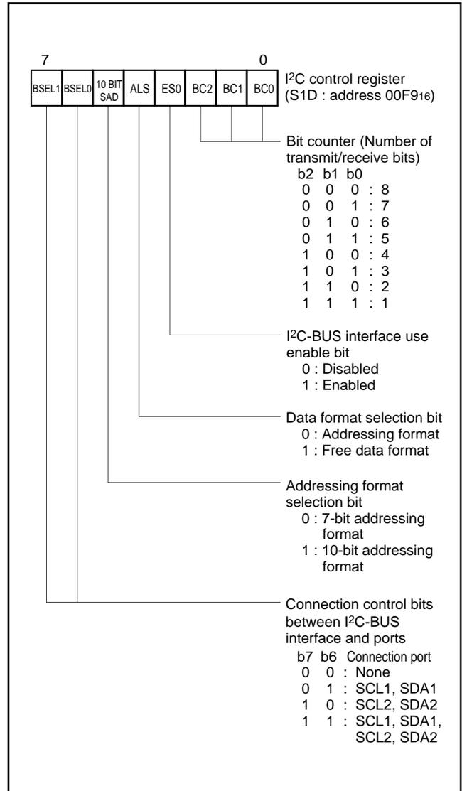
Fig. 43. Structure of I<sup>2</sup>C control register
