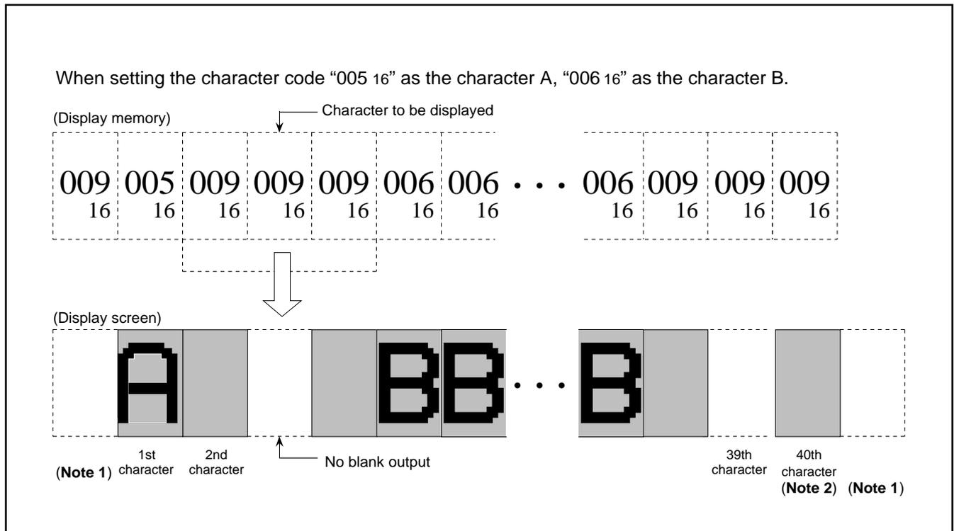
**Fig. 79. Display screen example of automatic solid space**
