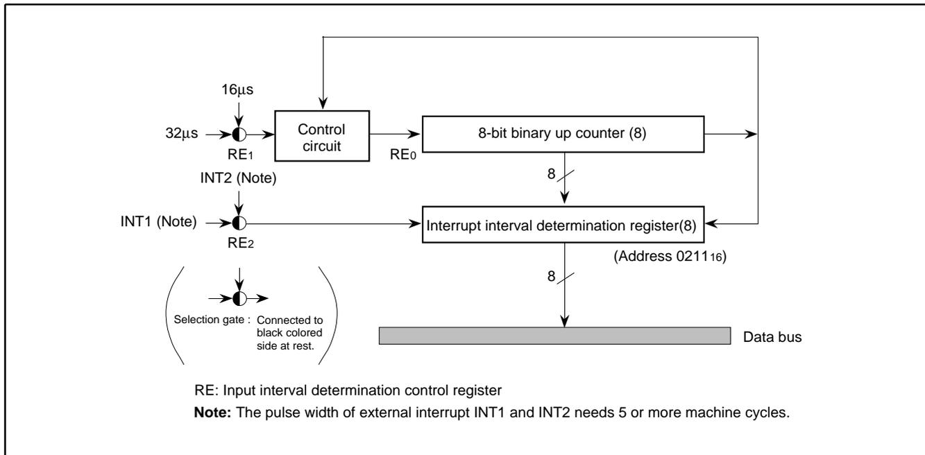
Fig. 86. Block diagram of interrupt interval determination circuit
