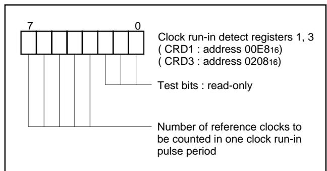
Fig. 36. Structure of clock run-in detect registers 1 and 3
