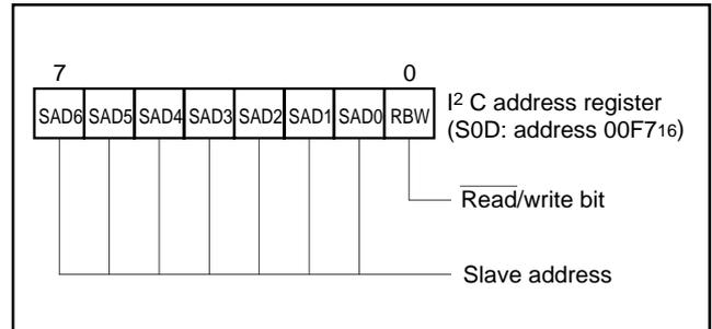
Fig. 40. Structure of I<sup>2</sup>C address register
