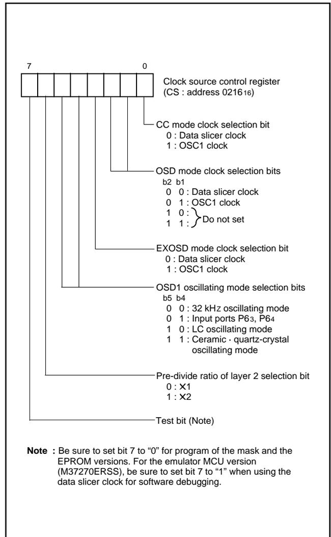
**Note :** Be sure to set bit 7 to "0" for program of the mask and the EPROM versions. For the emulator MCU version (M37270ERSS), be sure to set bit 7 to "1" when using the data slicer clock for software debugging.
