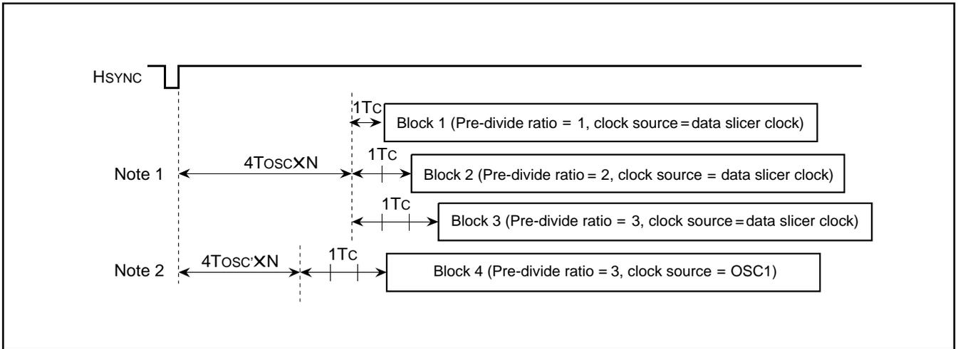
Fig. 60. Notes on horizontal display start position
