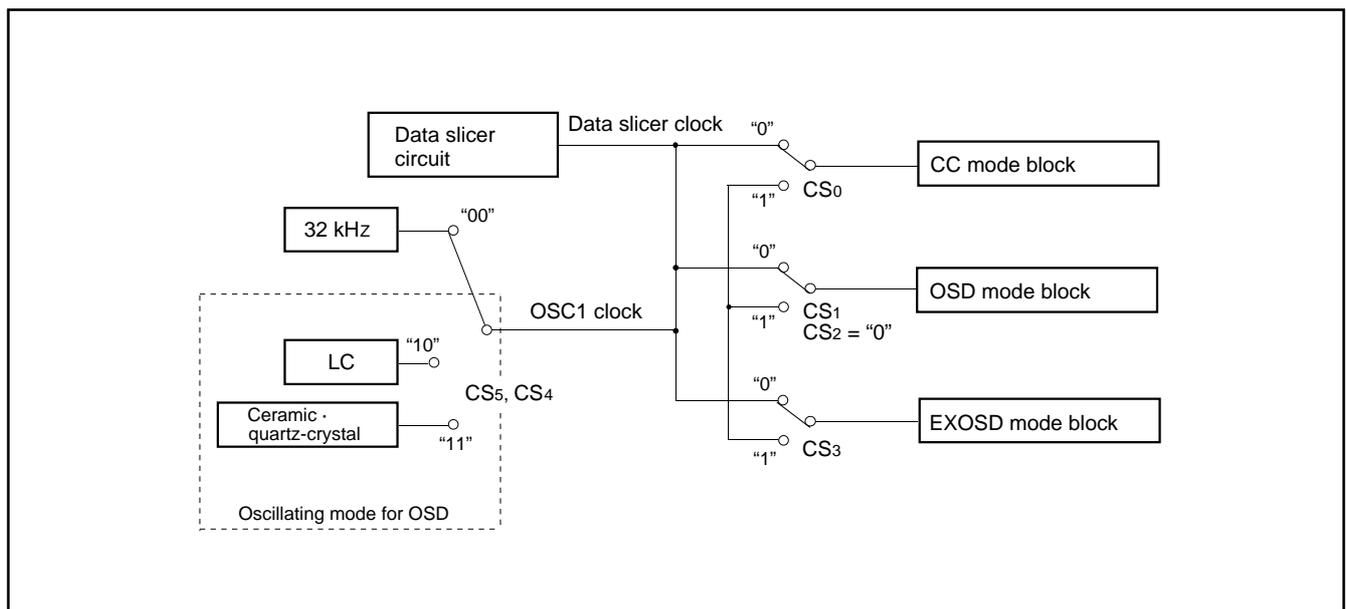
**Fig. 63. Block diagram of OSD selection circuit**
