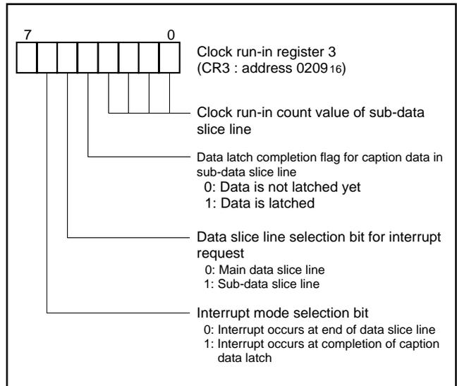
Fig. 34. Structure of clock run-in register 3
