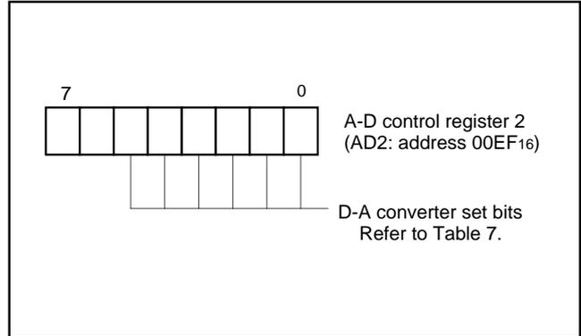
Fig. 29. Structure of A-D control register 2
