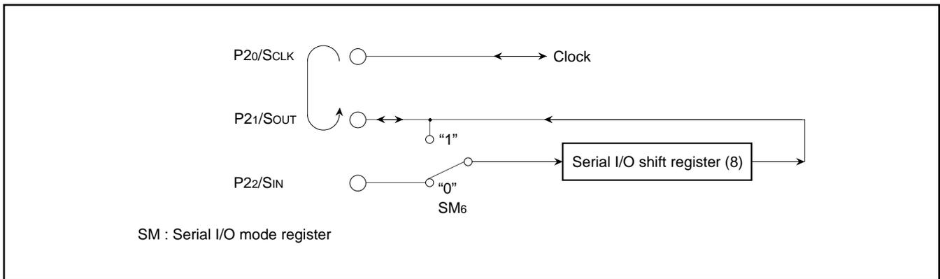
Fig. 11. Signals on serial I/O common transmission/reception mode
