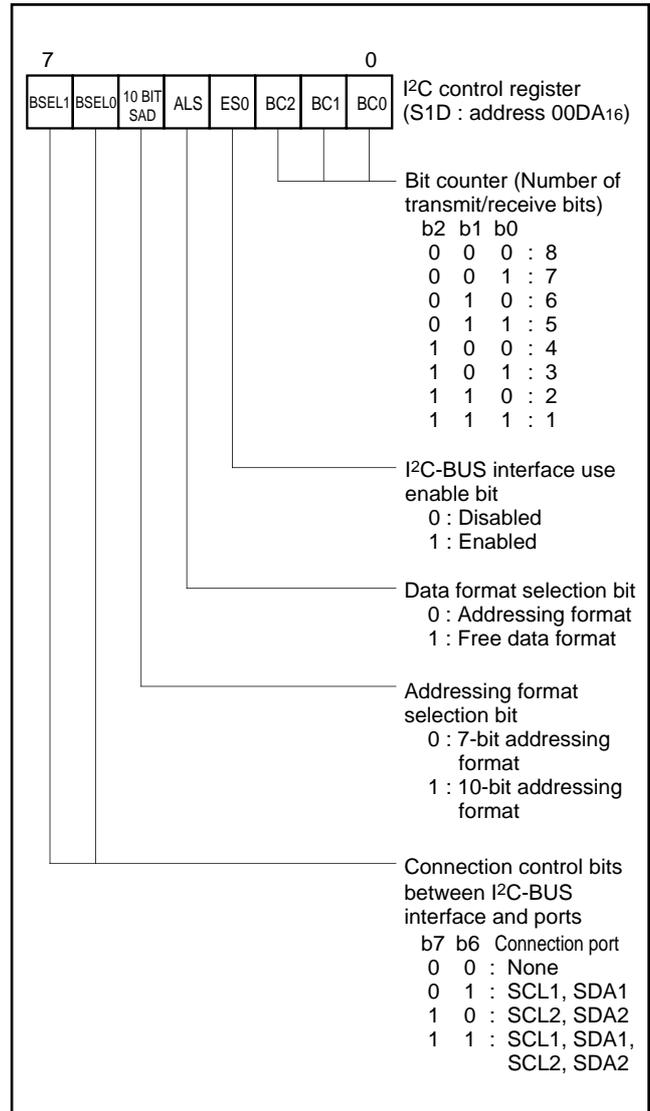
Fig. 16. Structure of I<sup>2</sup>C control register
