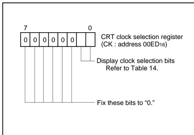
Fig. 48. Structure of CRT clock selection register
