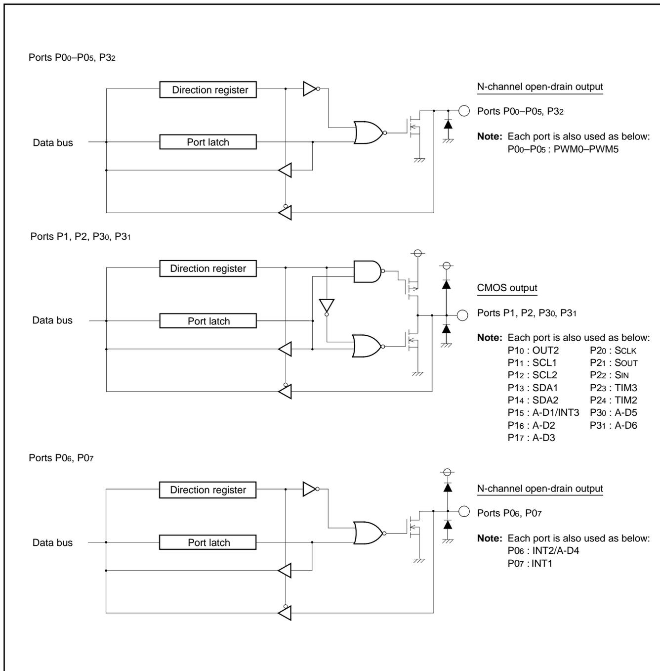
Fig. 52. I/O pin block diagram (1)
