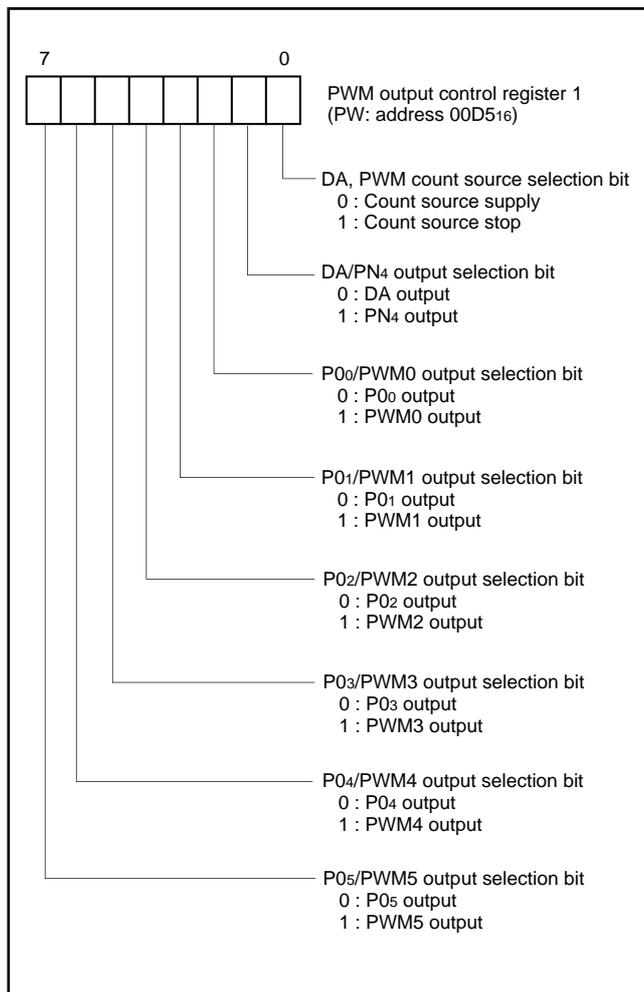
Fig. 26. Structure of PWM output control register 1
