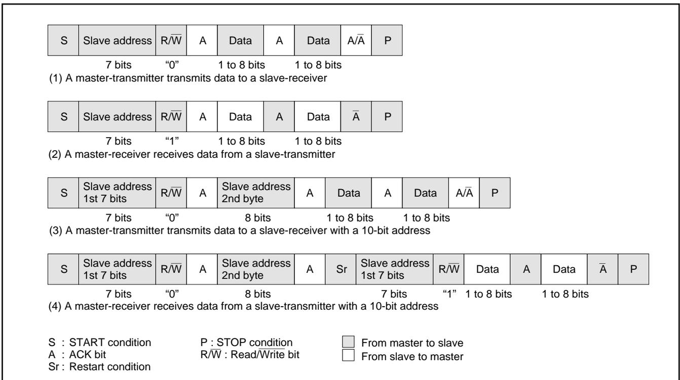
Fig. 22. Address data communication format
