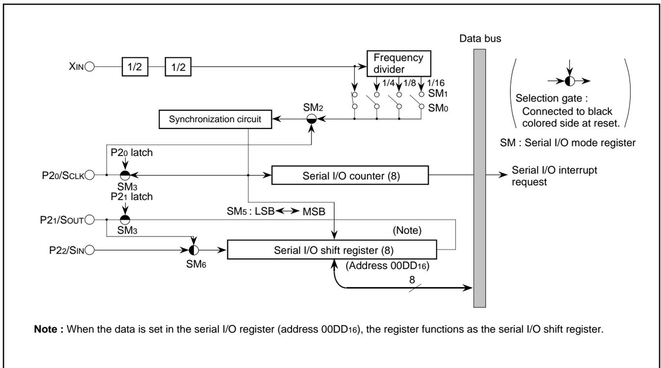
Fig. 8. Serial I/O block diagram
