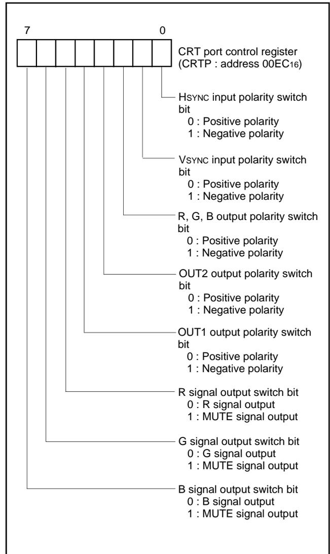
Fig. 46. Structure of CRT port control register
