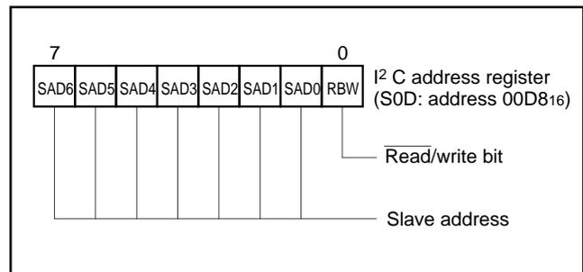
Fig. 13. Structure of I<sup>2</sup>C address register
