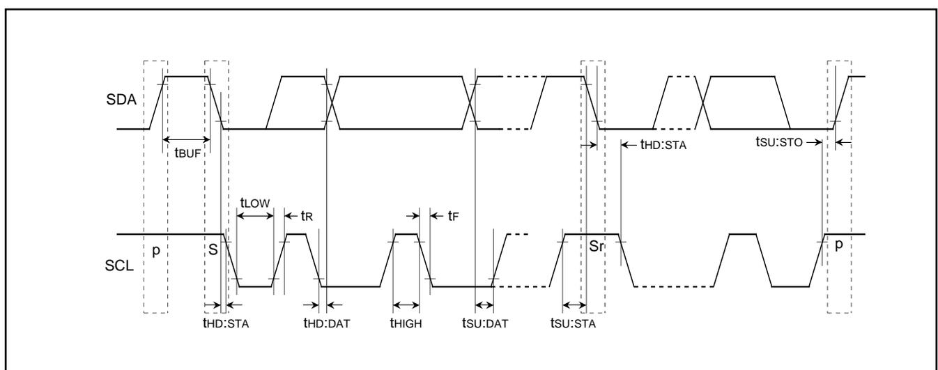
Fig. 59. Definition diagram of timing on multi-master I<sup>2</sup>C-BUS
