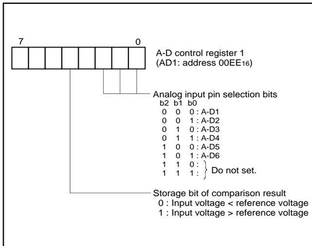
Fig. 28. Structure of A-D control register 1
