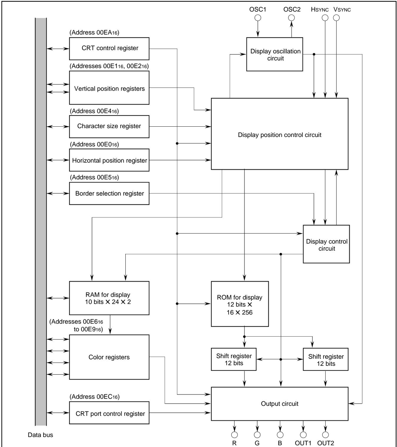
Fig. 33. Block diagram of CRT display control circuit
