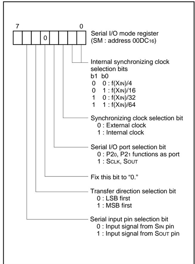
Fig. 9. Structure of serial I/O mode register
