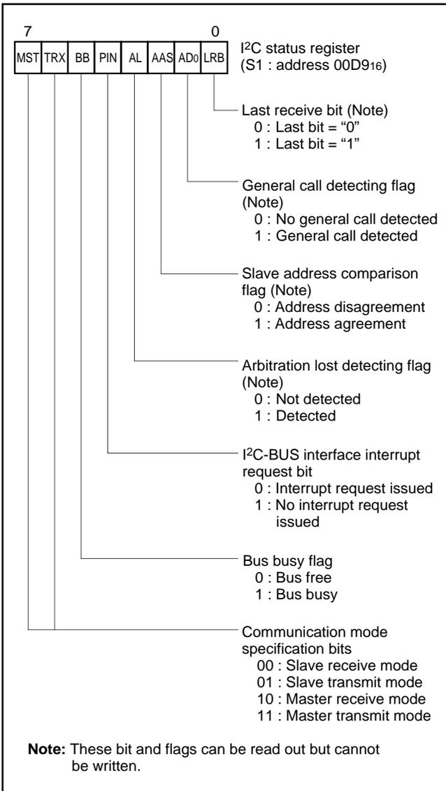
Fig. 17. Structure of I<sup>2</sup>C status register
