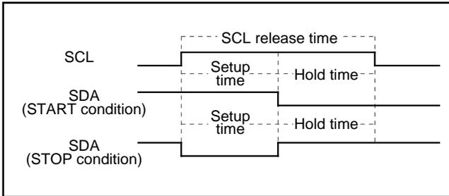
Fig. 21. START condition/STOP condition detecting timing diagram
