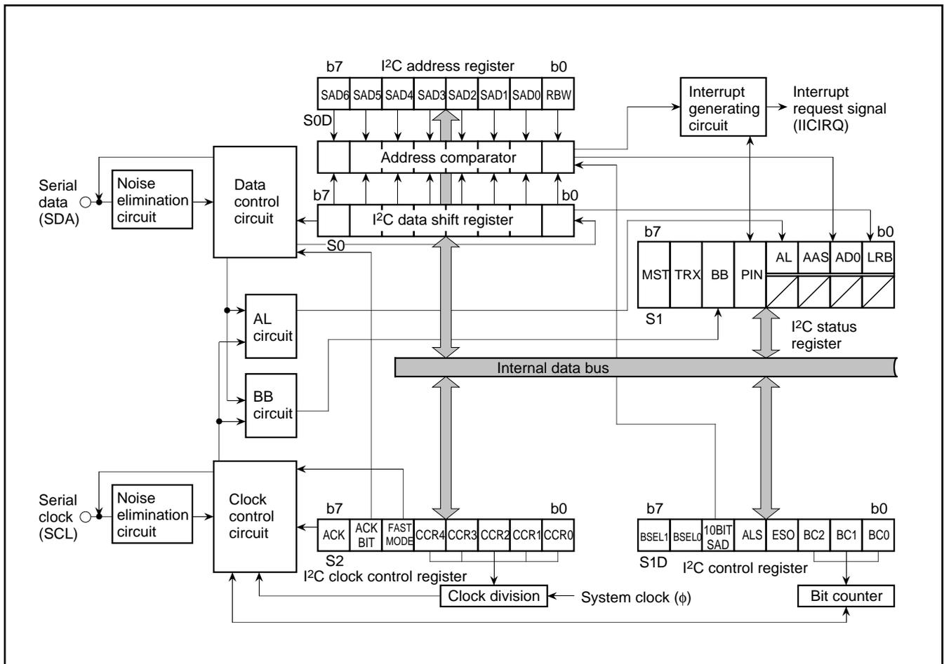
Fig. 12. Block diagram of multimaster I<sup>2</sup>C-BUS interface
