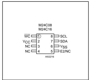
Warning: NC = Not Connected. Pin 5 is E2 for M24C08 and NC for M25C16.
