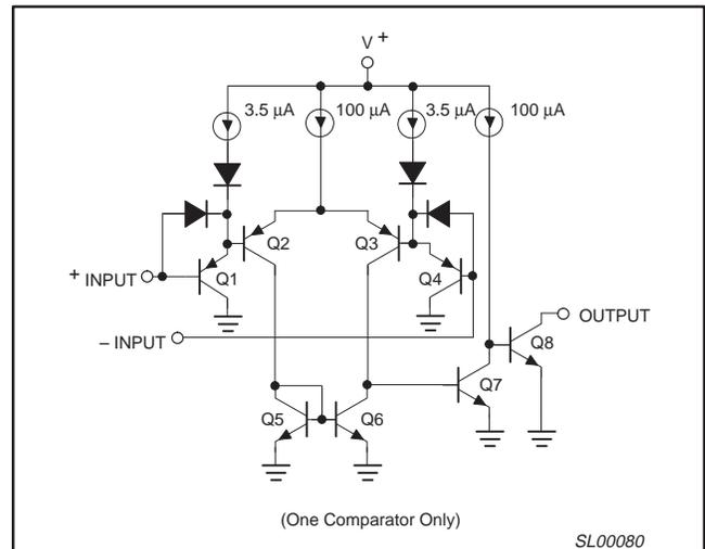
Figure 2. Equivalent circuit.
