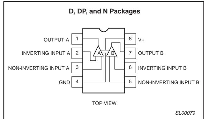
Figure 1. Pin configuration.
