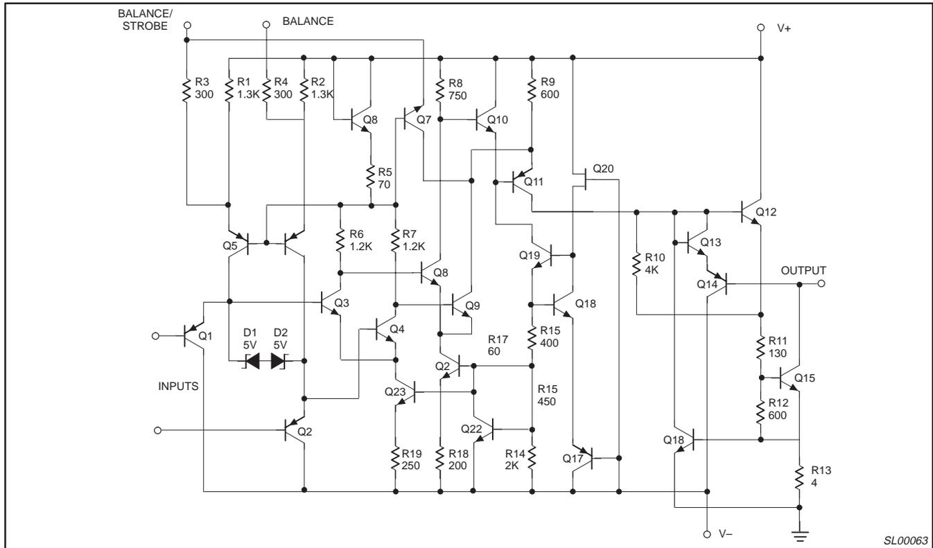
Figure 2. Equivalent Schematic
