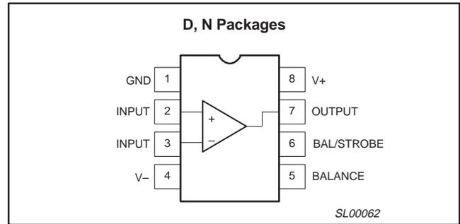
Figure 1. Pin Configuration
