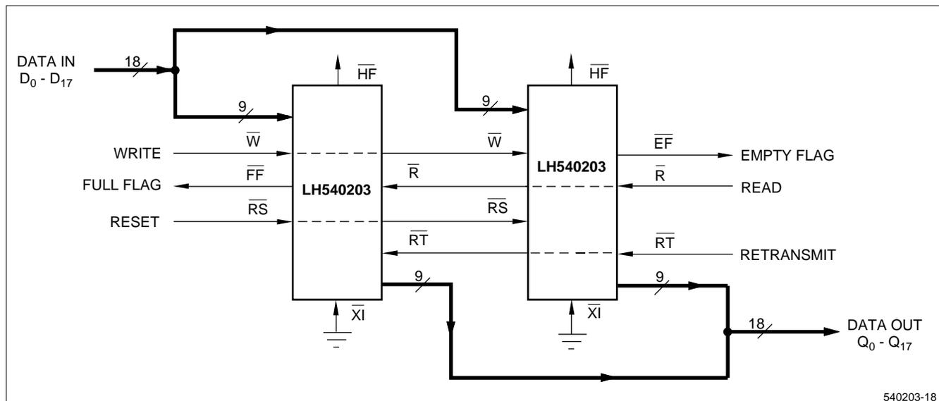
Figure 5. FIFO Word-Width Expansion (2048 × 18)
