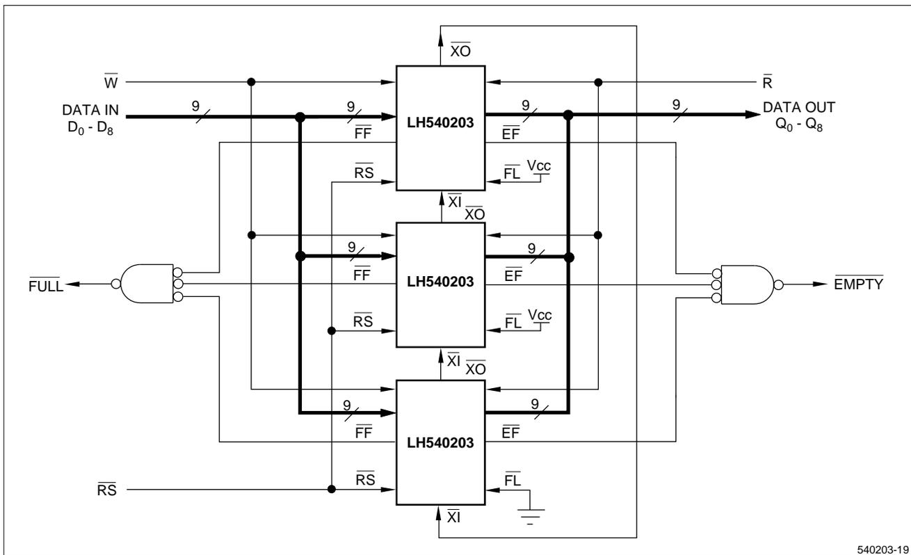
**Figure 6. FIFO Depth Cascading (6144 × 9)**
