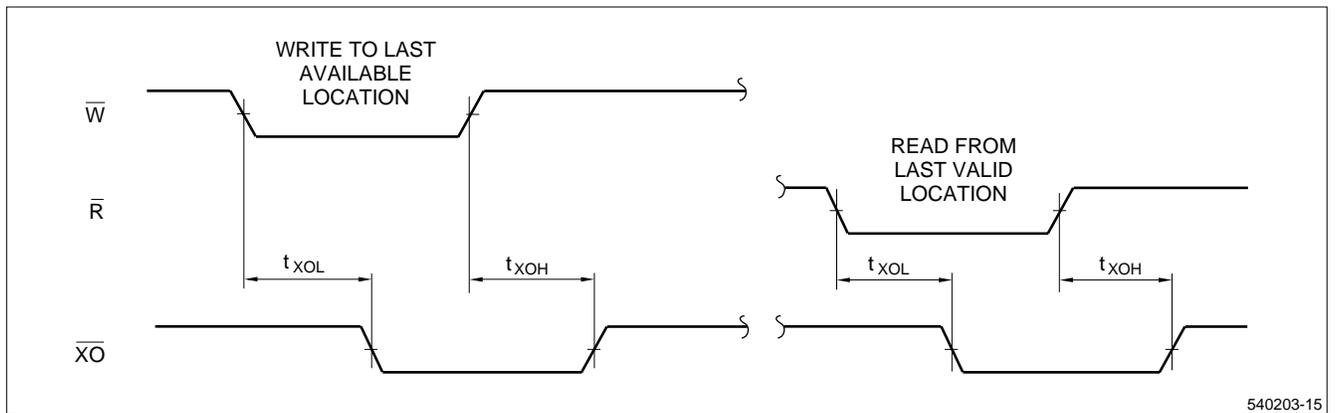
**Figure 20. Expansion-Out Timing**
