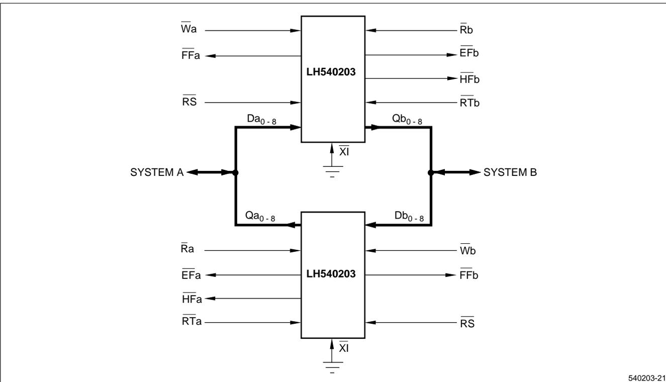
Figure 8. Bidirectional FIFO Operation
