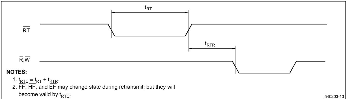
**Figure 19. Retransmit Timing**
