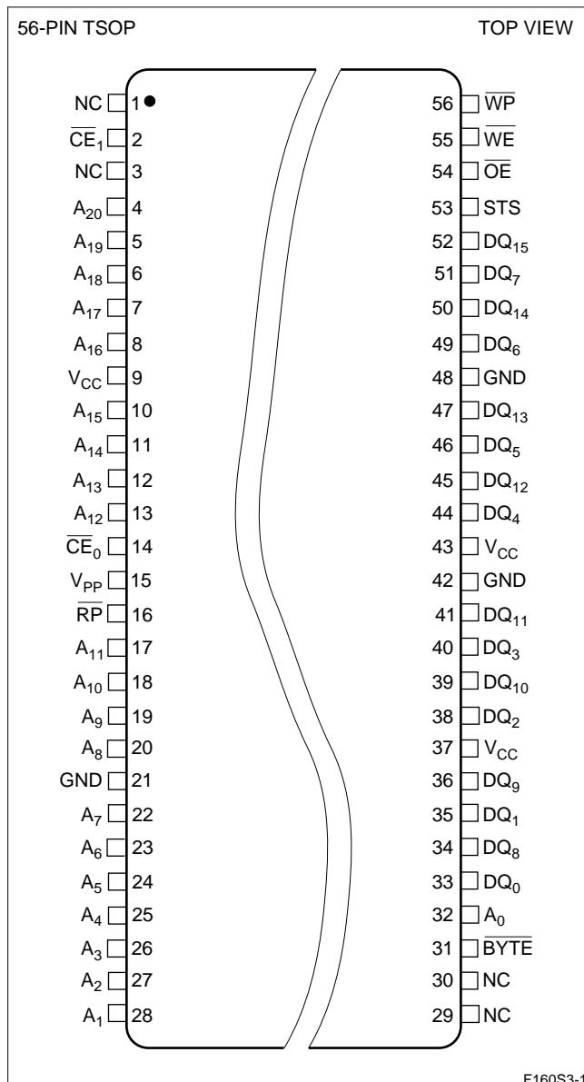
**56-PIN TSOP REVERSE BEND PINOUT**
