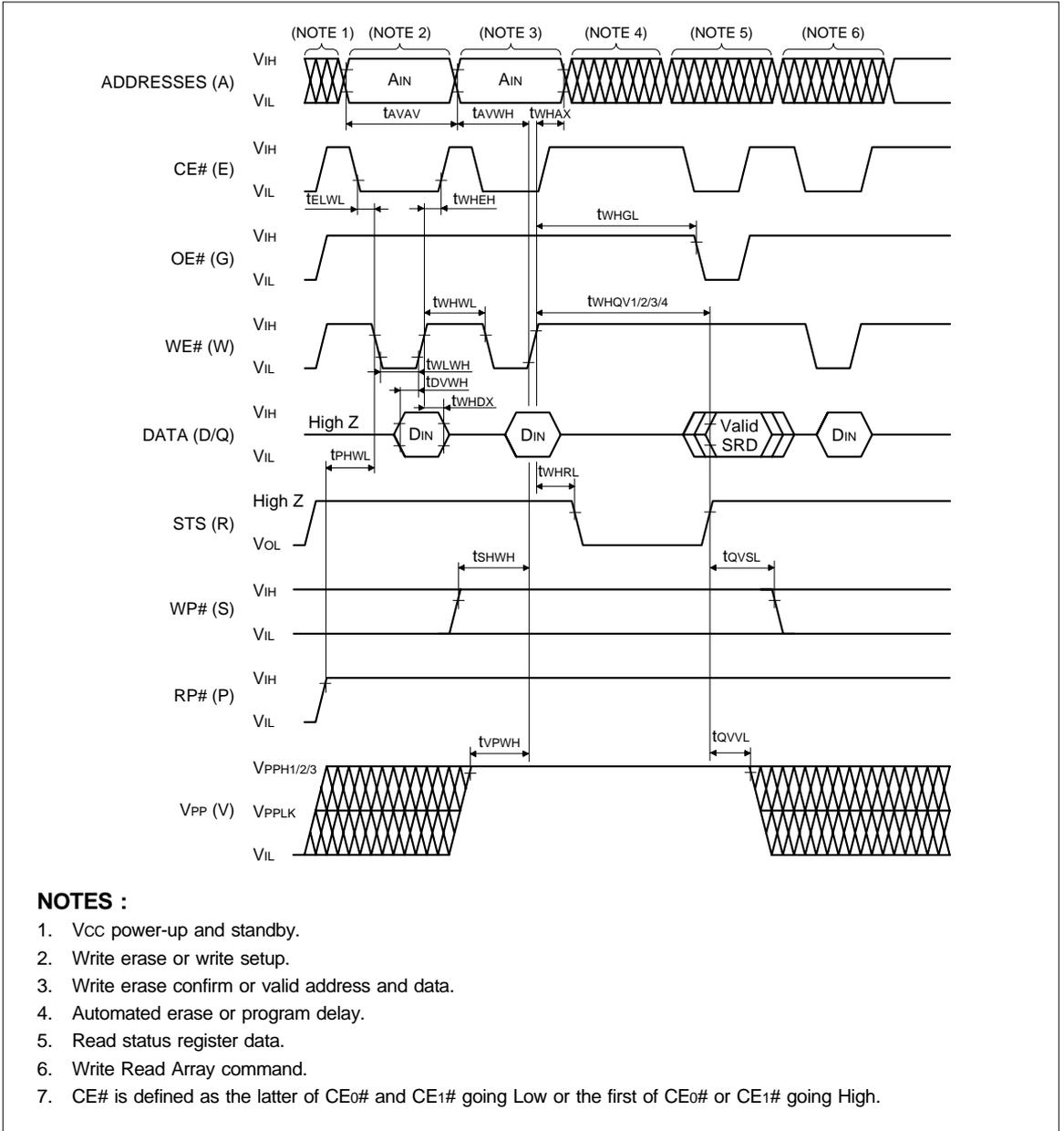
Fig. 17 AC Waveform for WE#-Controlled Write Operations
