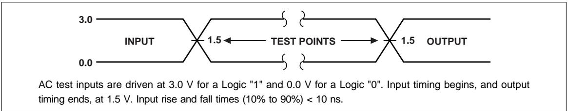
Fig. 13 Transient Input/Output Reference Waveform for  $V_{CC} = 3.3 \pm 0.3$  V
