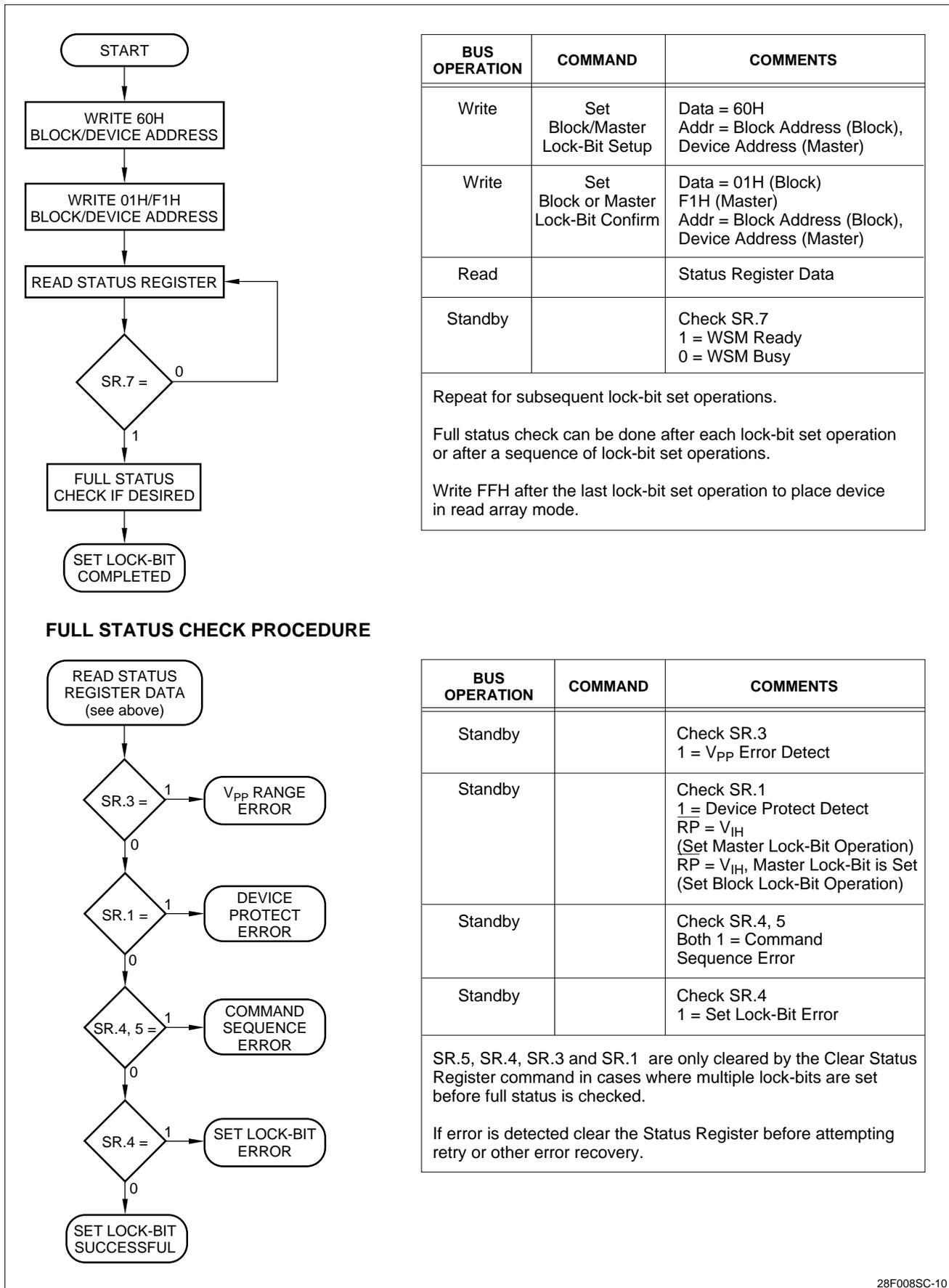
Figure 10. Set Block and Master Lock-Bit Flowchart
