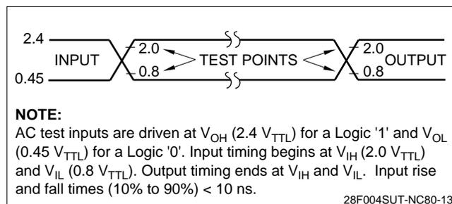
**Figure 14. Transient Input/Output Reference Waveform ( $V_{CC} = 5.0 V$ )**
