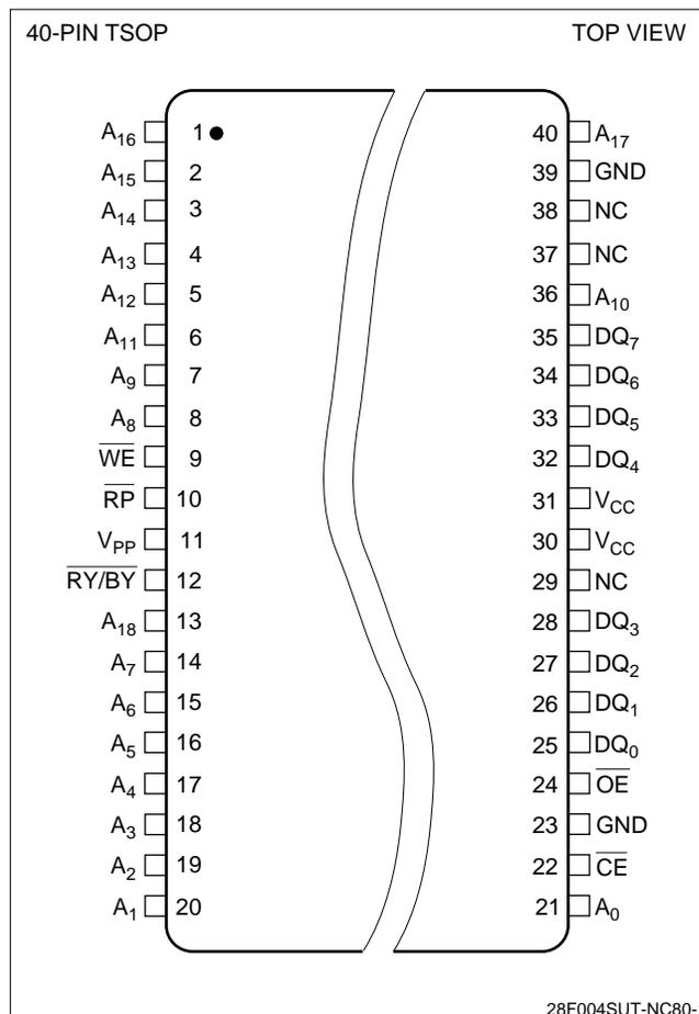
Figure 1. TSOP Configuration
