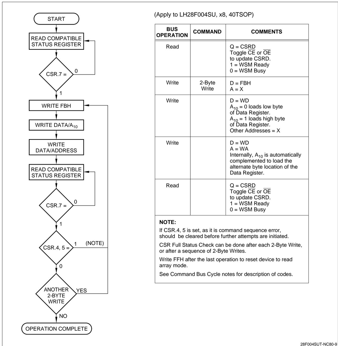
Figure 10. Two-Byte SerialWrites with Compatible Status Registers (LH28F00SU)
