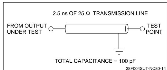
**Figure 15. Transient Equivalent Testing Load Circuit ( $V_{CC} = 5.0 V$ )**
