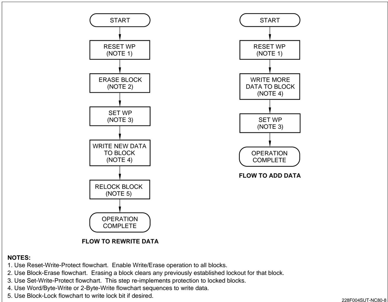
**Figure 9. Updating Data in a Locked Block**
