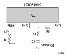
$R3 = 5.1 \text{ k}\Omega$ ,  $R4 = 200 \Omega$ ,  $R5 = 10 \text{ k}\Omega$ ,  $C3 = 0.1 \mu\text{F}$
