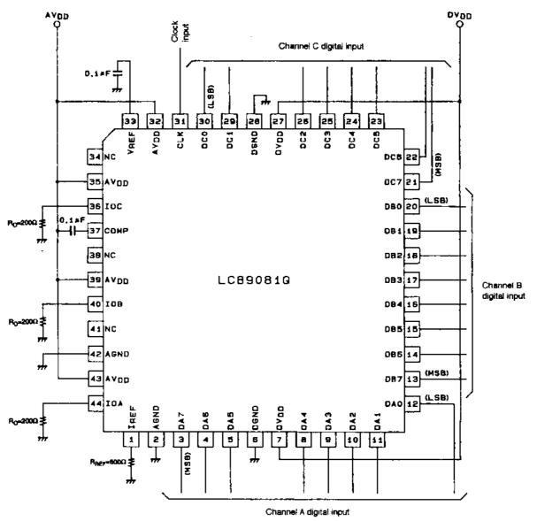
When operating at Fs = 30 MHz, Ro should be 75  $\Omega$  and RREF should be 600  $\Omega.$
