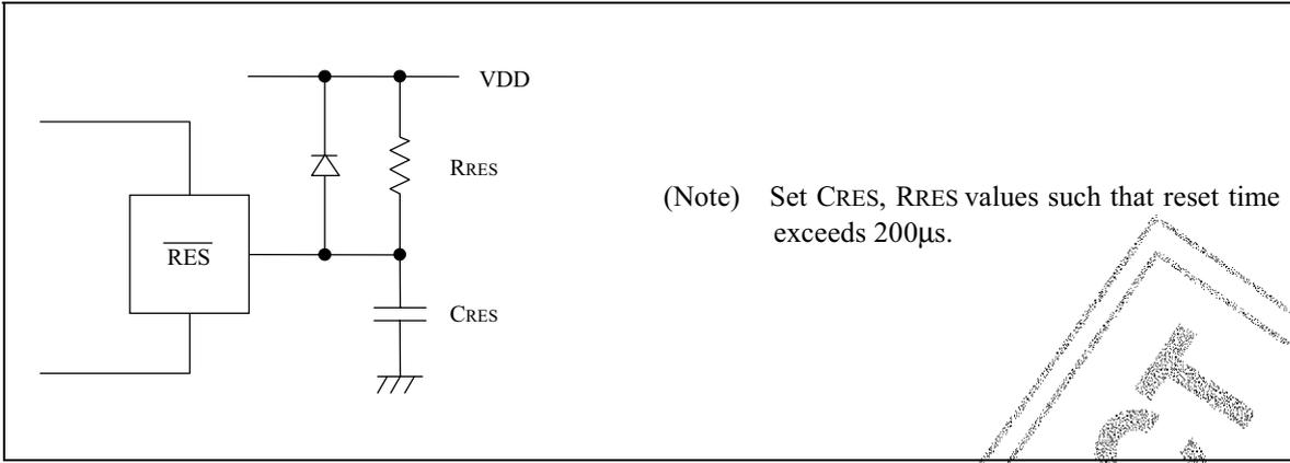
Figure 5 Reset circuit
