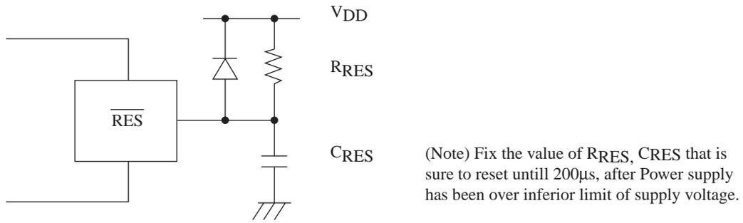
Figure 4. Reset circuit
