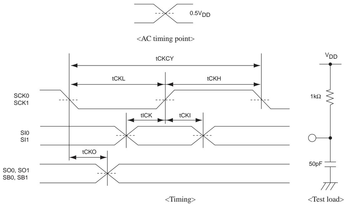
Figure 5. Serial input / output test condition
