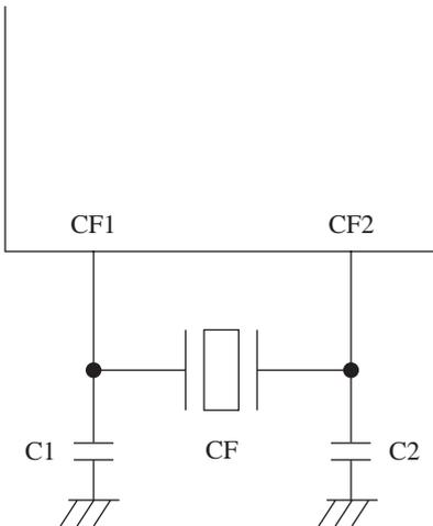
Figure 1. Main-clock circuit
