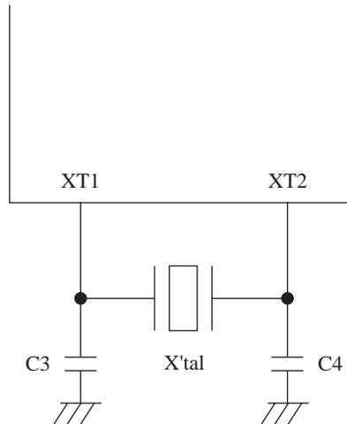
Figure 2. Sub-clock circuit
