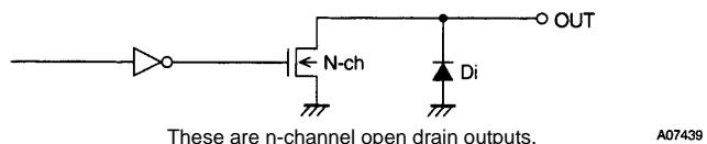
These are n-channel open drain outputs.
