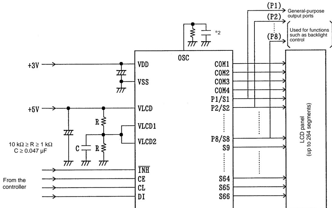
Note: \*2 When a capacitor except the recommended external capacitance ( $C_{osc} = 680 \text{ pF}$ ) is connected the OSC pin, we recommend that applications connect the OSC pin with a capacitor in the range 220 to 2200 pF.
