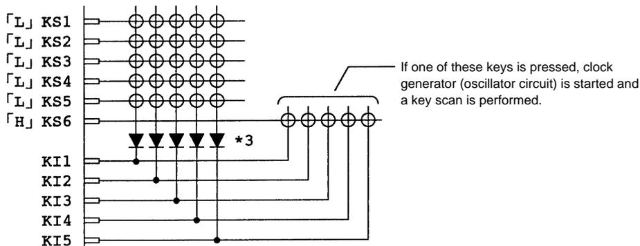
Note \*: These diodes are required to reliably recognize multiple key presses on the KS6 line when the IC is set to sleep mode with only KS6 set to high as in the example above. That is, they prevent incorrect recognition of key presses due to sneak currents arising from simultaneous presses of keys on the KS1 through KS5 lines.
