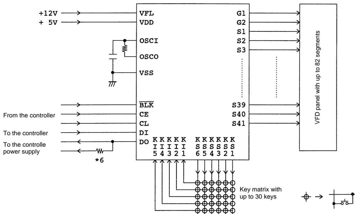
Note \*: Since DO is an open-drain output, a pull-up resistor is required. Select a value in the range 1 to 10 kΩ that is most appropriate for the capacitance of the external lines so that the waveform is not distorted.
