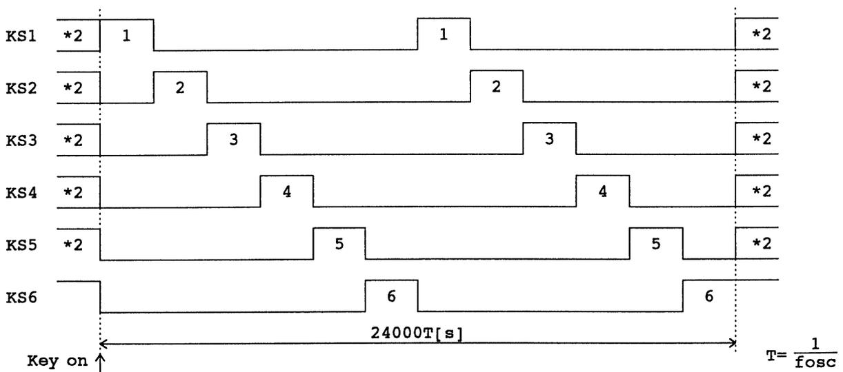
Note \*: The high-level and low-level states in sleep mode are set according to the control data S0 and S1. Key scan output signals are not output from pins set to the "L" state.
