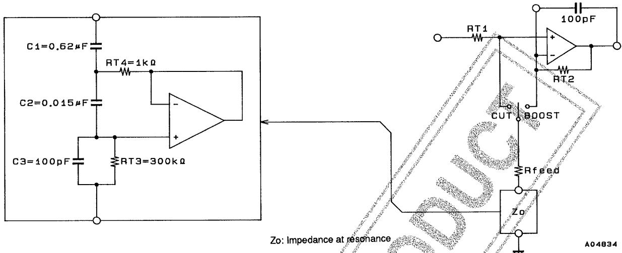
The output noise can be improved by about 6 dB by providing an external impedance at resonance of  $Z_o$  and adding the capacitor  $C_3$  with a value of about 100 pF. An even larger noise reduction effect can be acquired by using a low noise operational amplifier in the external circuit.
