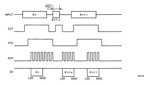
When the data output is disrupted due to input clock displacement.
