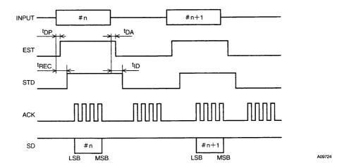
When the DTMF signal (#n) is split due to, for example, the burst signal
