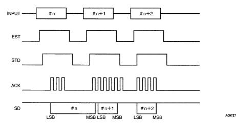
Data is output from the SD pin after 4 pulses are input to the ACK pin. However, note that if 5 or more pulses are input between one rising edge on the EST pin and the next rising edge on the EST pin, the fifth and later pulses will be ignored.
