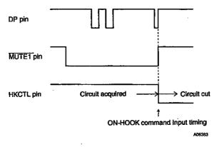
• The following gives the timing for an ON-HOOK command during tone dialling.
