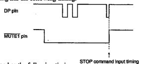
A stop command during tone dialling has the following timing.
