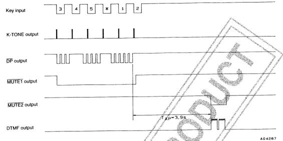
If a DTMF key operation is performed during dialing pulse output (including IDP), the K-TONE signal will be output continuously while keys are pressed. Then, after the pulse dialing completes, the LC737212/M will pause for 3.9 seconds and then output the DTMF signals.
