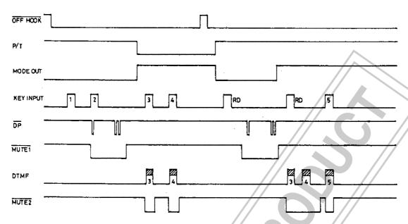
The mode after completion of redialing is set again by the P/T SW position provided when redialing is completed.
