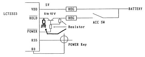
2. When an external power switch is used (when the diode matrix POWSEL setting is 0 or 1)
