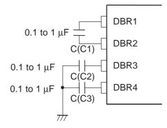
Notes: \*1. The capacitors C(1), C(2), and C(3) must be connected to the DBR pins.
