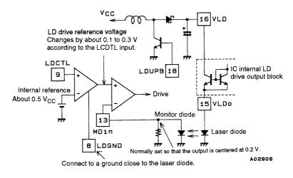
First, when  $V_{CC}$  is adequately high (about 2.5 V or over) the laser diode is driven by the system consisting of  $V_{CC}$ , an inductor and a Schottky diode without driving LDUPB. Then, when  $V_{CC}$  falls and  $V_{LD} - V_{LDO}$  become under about 0.3 V, LDUPB is driven,  $V_{LD}$  is stepped up, and the circuit is controlled so that  $V_{LD} - V_{LDO}$  is held at 0.3 V (typical).
