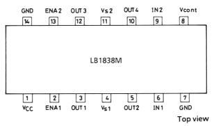
Note: Both GND pins should be connected to ground.
