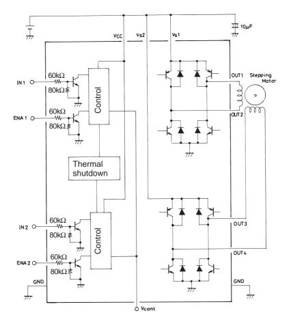
Note: As long as the voltages applied to  $V_{CC}$ ,  $V_S1$ ,  $V_S2$ , ENA1, ENA2, IN1, and IN2 are within the limits set by the absolute maximum ratings, there are no restrictions on the relationship of each voltage level in comparison with the others (regarding which is higher or lower). (ex.  $V_{CC} = 3$  V,  $V_S1$ , Z = 2 V, ENA = IN = 5 V)
