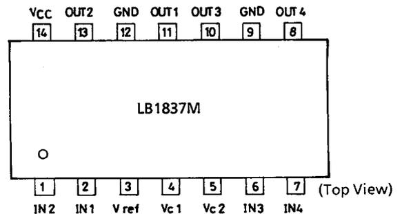
Note: Both GND pins must be grounded.
