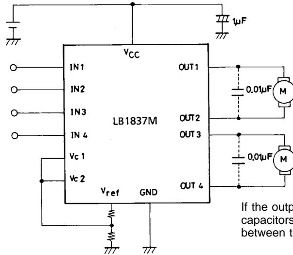
If the outputs oscillate, insert capacitors of 0.001 to 0.1  $\mu\text{F}$  between the outputs.
