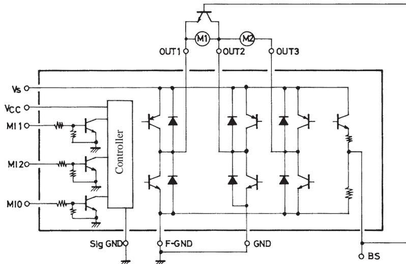
Note) Use one of the FRAME-GND pins for grounding. When the Cu-foiled side is soldered, heat radiation can be more improved.
