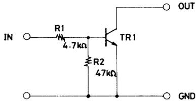
Equivalent Circuit Block Diagram
