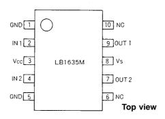
Note: both ground pins must be grounded.
