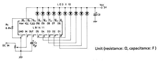
Constant current of D output is determined by R1. 1mA typ. at  $6.8k\Omega$
