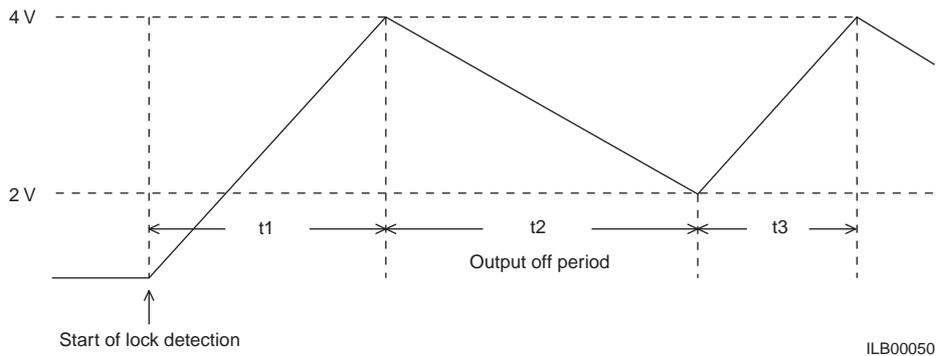
The following formula gives the time, t1, from the point the motor speed is locked until the output is turned off.
