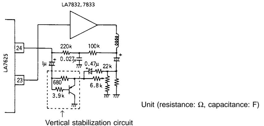
Vertical output IC (LA7837, 7838) connection circuit example
