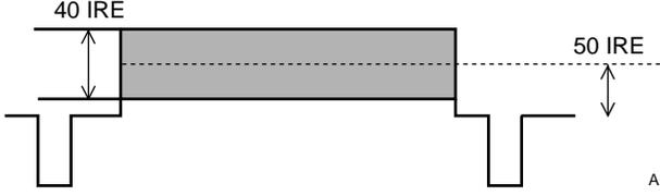
A10059     | 45.75 MHz<br>87.5% video modulation<br>Sweep signal<br>(APL: 50 IRE, sweep signal level: 40 IRE) |
