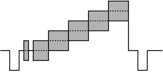
A10058       | 45.75 MHz<br>87.5% video modulation<br>10-step waveform<br>(subcarrier: 3.58 MHz)                |
