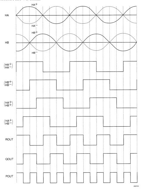
Note: When the sled motor rotation direction changes (that is, when the HA and HB phase relationship changes), the R-OUT and Q-OUT phase relationship changes and the direction can be detected from that phase. The motion distance and position are detected from P-OUT.
