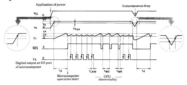
Note : Edge-triggered at the point indicated by the arrow of  $C_K$  signal.
