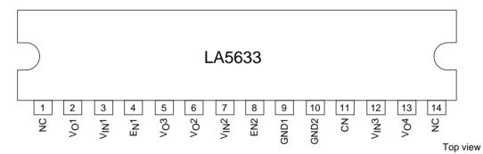
Note: NC pins must not be used (Pins 1 and 14 in the pin assignment figure.)
