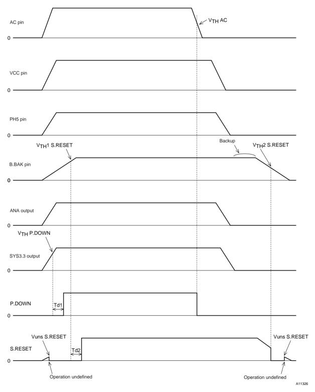
Note: The S.RESET output has an undefined operating state, so care is required in application design.
