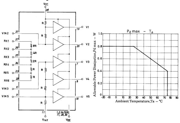
Note : Use the IC so that  $V_{RX1} \!\!\ge\!\! V_{RX2} \!\!\ge\!\! V_{RX3} \!\!\ge\!\! V_{RX4} \!\!\ge\!\! V_{RX5} \!\!\ge\!\! V_{RX6}$  is obtained.
