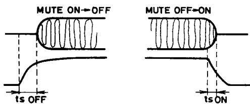
The mute ON/OFF switching waveforms are shown in the figure above. The settling time  $t_s$  is determined by the capacitor  $C_r$  connected to pin 16. The recommended value of  $C_r$  is 1  $\mu\text{F}$ . If the value used is less than 1  $\mu\text{F}$ , pop noise will increase.
