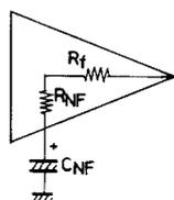
$$A_{vf} = \frac{R_f}{\left( R_{NF} + \frac{1}{j\omega C_{NF}} \right)}$$
