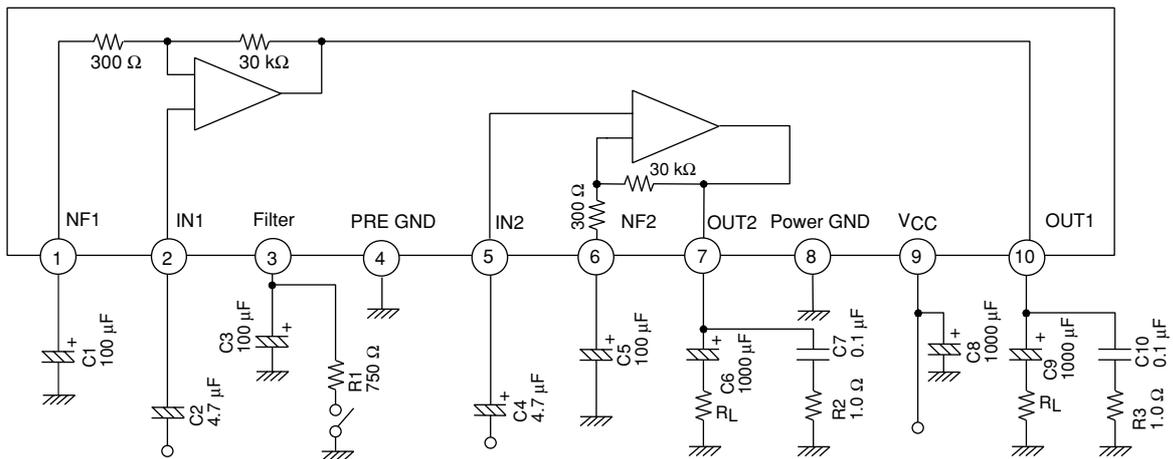
\* For Muting, add a resistor between pin 3 and GND. 750  $\Omega$  for the LA4266/67/68, 200  $\Omega$  for the LA4276/77.
