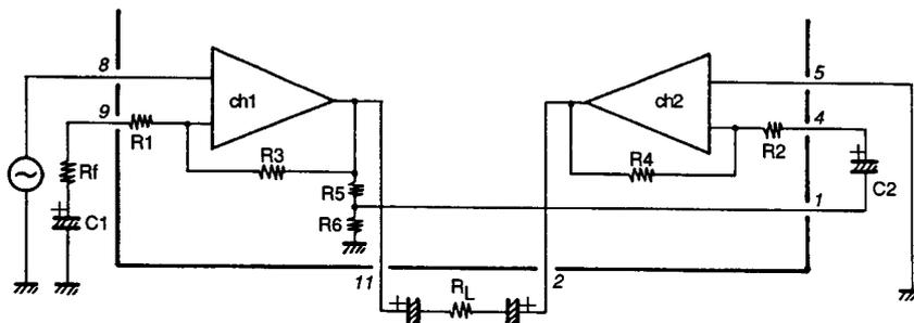
The output of ch1 is divided with R5, R6 and led to pin 1 and then inputted to ch2. Since the attenuation degree (R5/R6) of ch1 output and the amplification degree (R4/R2 + R6) of ch2 are fixed at an equal value, the ch2 output is in opposite phase with the ch1 output. Therefore, the total voltage gain gets apparently 6 dB higher than the voltage gain of ch1 alone and is determined by the following equation.
