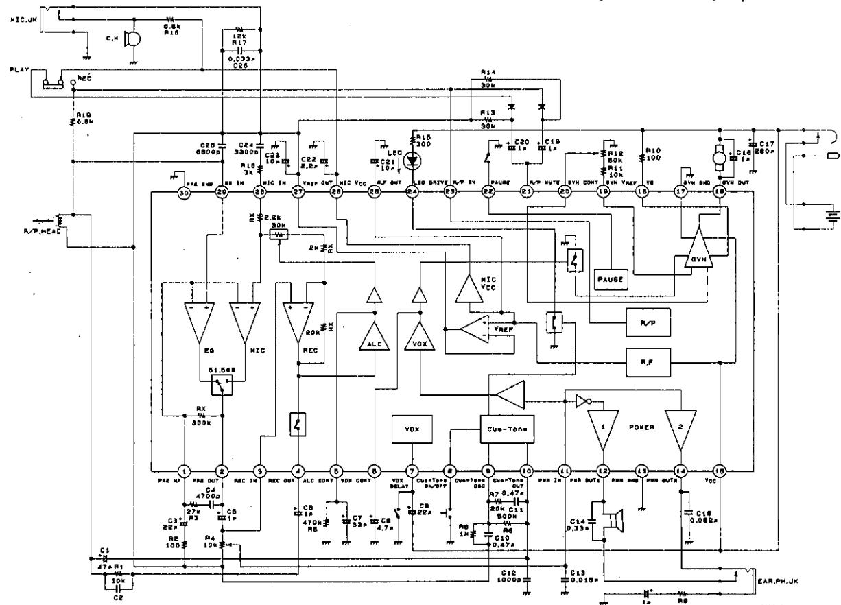
**Pin Assignments and Equivalent Circuits**[ $V_{CC}=3.0V$ ]
