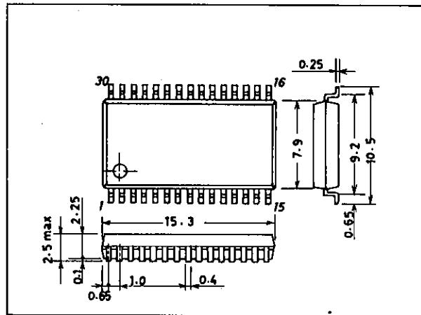
The LA4167M is a record/playback system IC supporting microcassette and compact cassette recorders. This is a high-performance IC that has on-chip a governor circuit for motor control, a voice sensor circuit that detects sounds and switches the motor on and off, and a cue-tone circuit for instantly finding the desired segment to play back.
