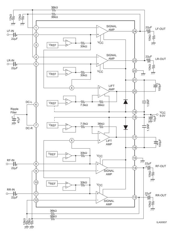
Note: We recommend using resistors with tolerances of 1% or better for the 12  $k\Omega$  and 36  $k\Omega$  feedback resistors.
