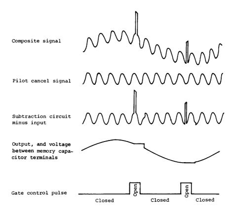
Note: The pilot cancel signal is given as sinusoidal in this explanation, but in the actual specimen application circuit, pilot cancel is performed by a triangular wave.
