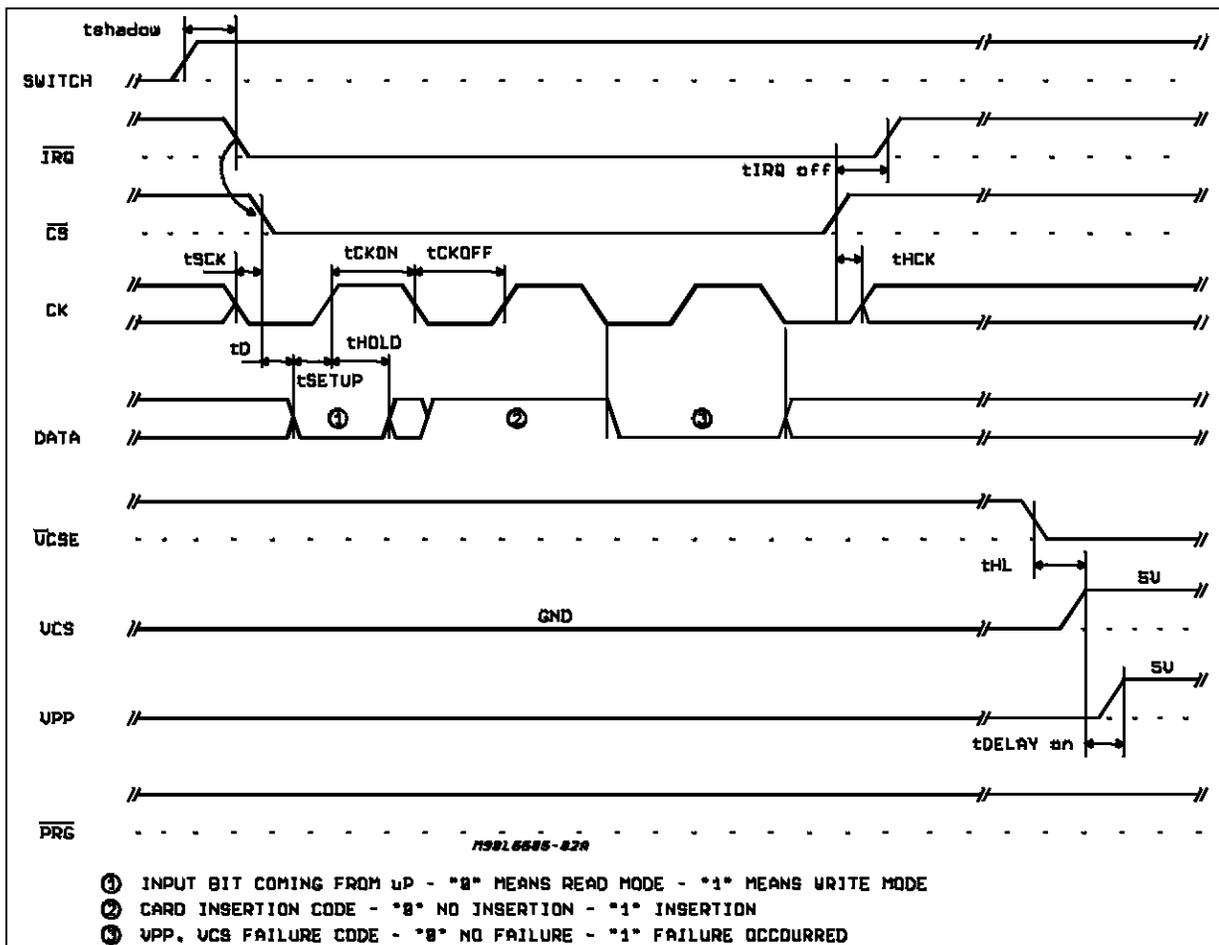
Failure could be overtemperature over the 2 regulators (VPP, VCS).
