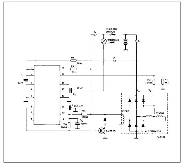
The device is able to withstand all the voltage transients mentioned in ISO DP7637/1. If voltage transients more severe than the above ISO standard have to be withstood, an external protection device
