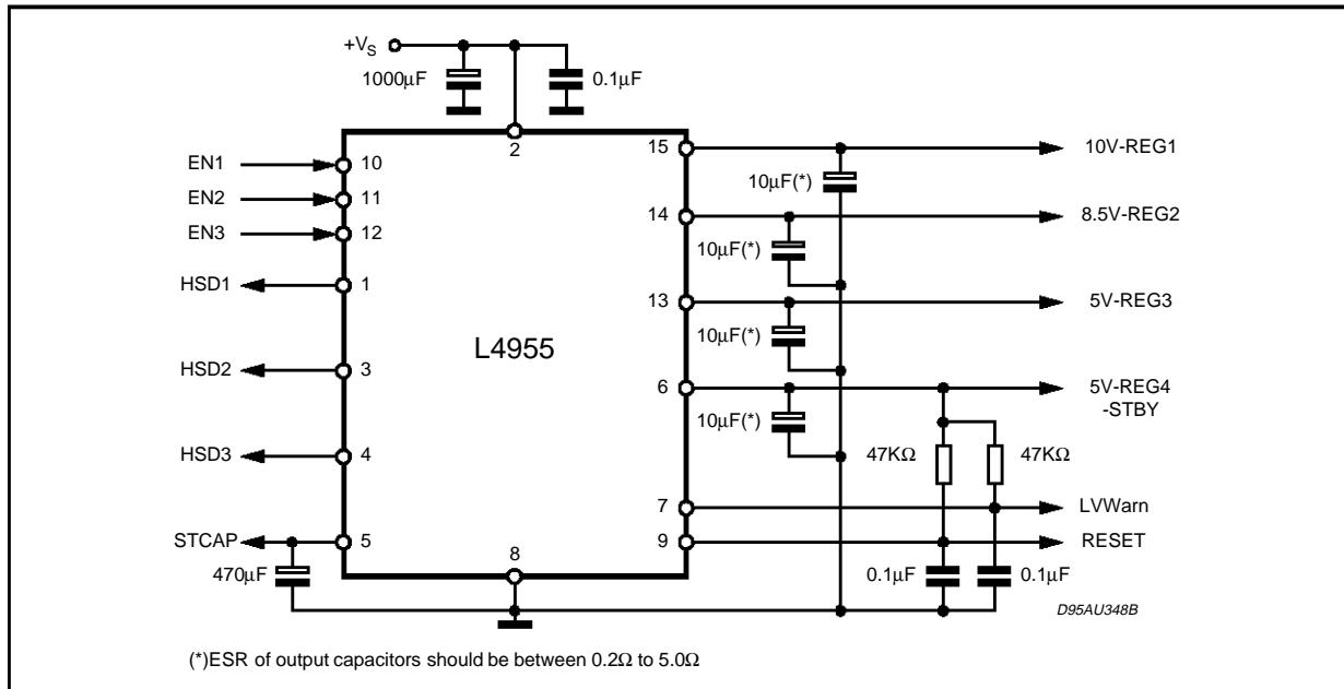
**ELECTRICAL CHARACTERISTICS** (Refer to the application circuit,  $V_S = 14.4V$ ;  $T_{amb} = 25^\circ C$ ;  $I_{OUT10} = 5mA$ ;  $I_{OUT8.5} = 5mA$ ;  $I_{OUT5} = 5mA$ ;  $I_{OUT5\ ST-BY} = 0.5mA$ ;  $R_{HSD1} = 16\Omega$ ,  $R_{HSD2,3} = 107\Omega$ , unless otherwise specified.)
